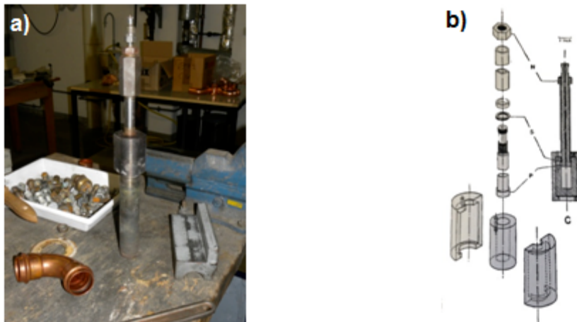
Fig. 12 – a) Pressure vessel used for the experiment and b) sketch of the pressure vessel (modified after Tuttle 1949).
