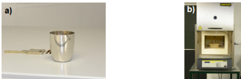
Fig. 9: a) platinum crucible used for the syntheses and b) furnace used for the heating of the samples.
