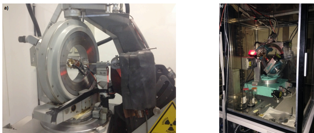
Fig. 26 – a) Philips PW1100 diffractometer at the University of Pavia equipped with the old design of the microfurnace and b) HUBER four-circle diffractometer at the University of Pavia equipped with the new design of the microfurnace. Both the diffractometers are equipped with a point detector.
