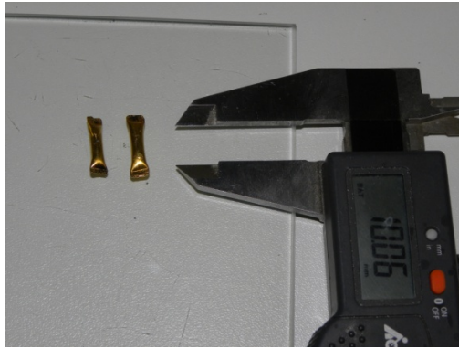
Fig. 13 – Gold capsules used for the synthesis of garnets in hydrothermal conditions.
