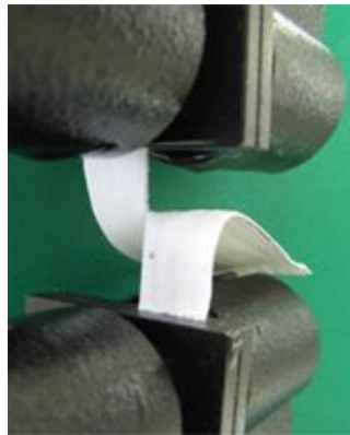
Figure 3 Tear resistance testing [16].
