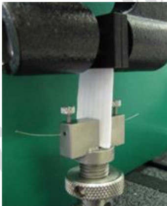
Figure 2 Suture retention testing [16].
