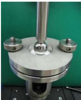
Figure 6 Ball burst testing [16].
