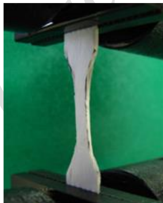
Figure 4 Uni-axial tensile testing [16].
