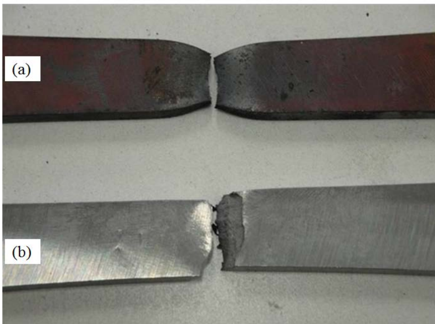
Fig. 7: Fracture surface of plain specimen tested at 650^{\circ}\text{C} (a) ( \Delta\sigma=140 MPa, N=284049 ), and room temperature (b) ( \Delta\sigma=900 , N=155000 )
