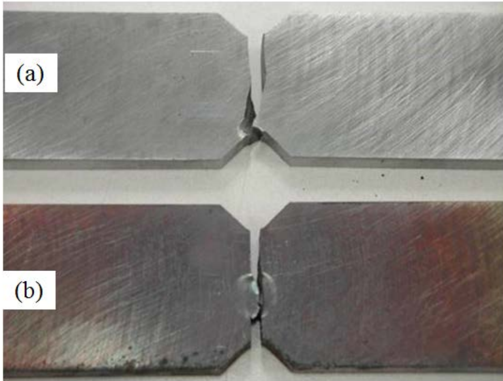
Fig. 9: Fracture surfaces of the V-notched specimens tested at room temperature (a) ( \Delta\sigma=250 MPa, N=295000 ) and high temperature (b) ( \Delta\sigma=100 MPa, N=304000 )
