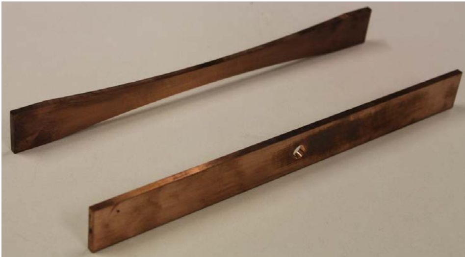
Fig. 9: Hour-glass shaped specimen and notched specimen
