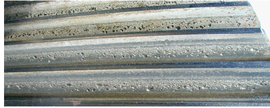
FIGURE 1.2: Dedendum wear of a hardened gear.
