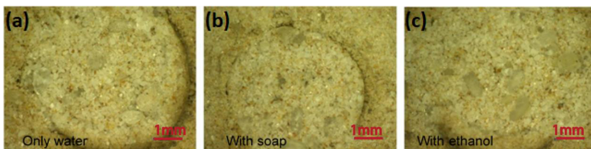
Figure 3.15. (a) water droplet on BdZ printing mix; (b) water plus soap droplet on BdZ printing mix; (c) water plus ethanol droplet on BdZ printing mix.
