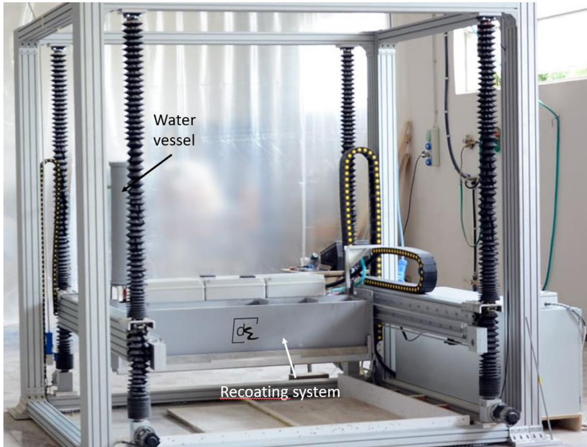
Figure 3.13. Actual configuration of the printer with water vessel and recoating system. [95]
