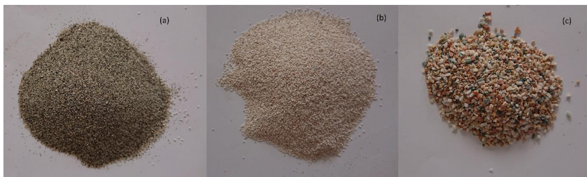
Figure 2.16. Desamanager aggregates, (a) River Po Sand, (b) Bianco di Zandobbio dolomite, (c) Marble granules.
