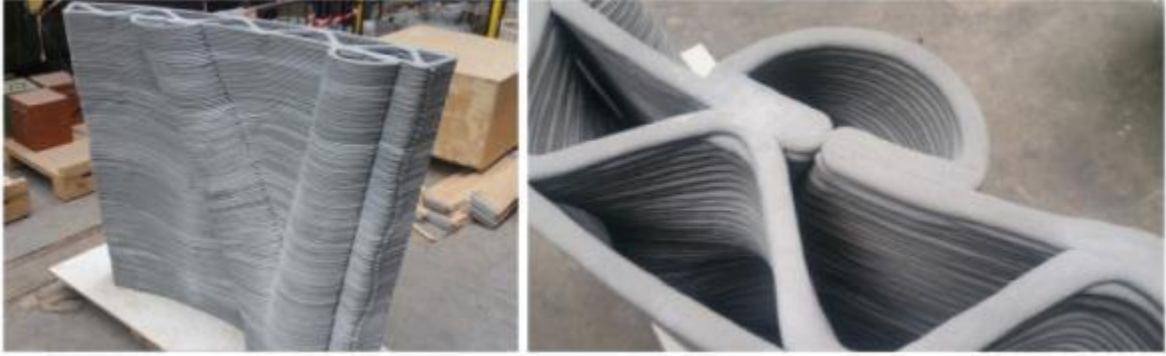
Figure 30. UHPC printed wall elements. [46]
