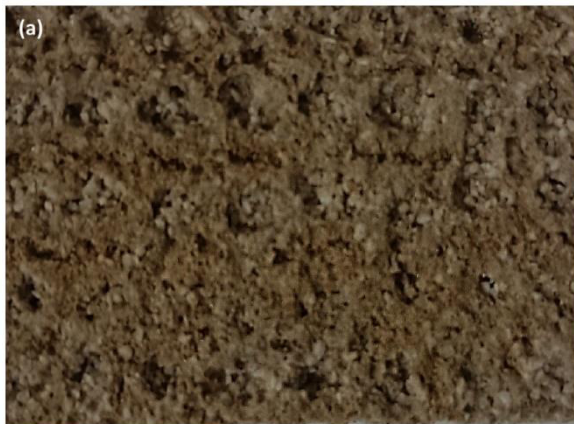
Figure 3.12. (a) Interface between layers from the top and (b) the voids created from water droplets from the section.
