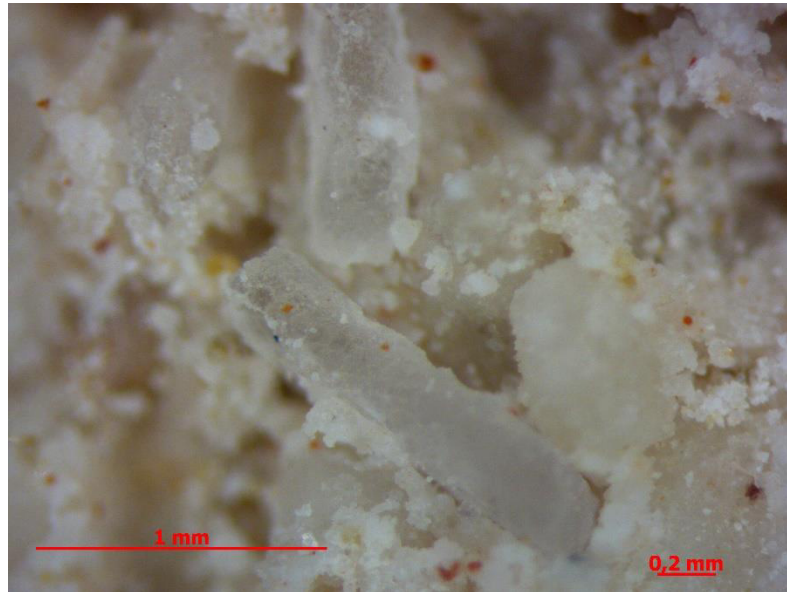
Figure 4.10. Unreacted MKP crystal.
