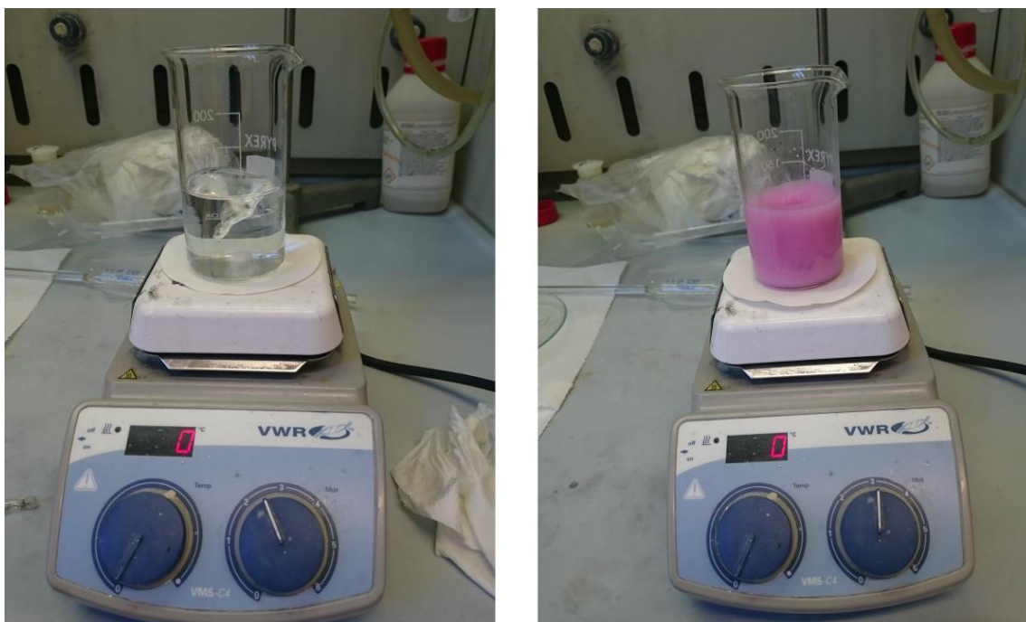
Figure 4.1. Activity test: on the left the solution before the addition of MgO, on the right the same after the change of the indicator during the neutralization reaction
