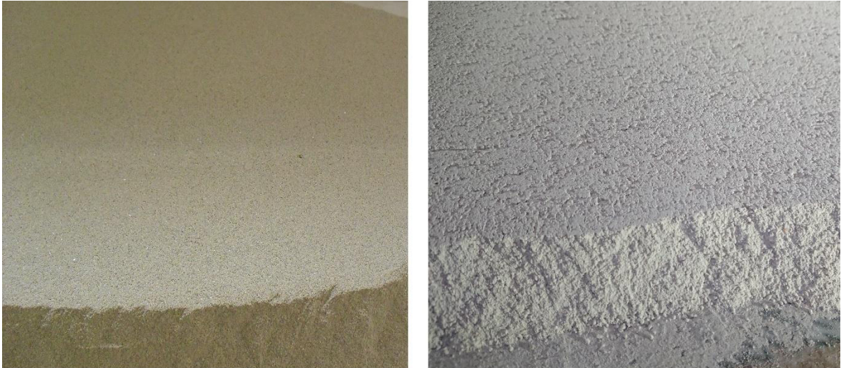
Figure 4.8. Quality of different particle size bed; on the left the fine powder; on the right the coarse powder.
