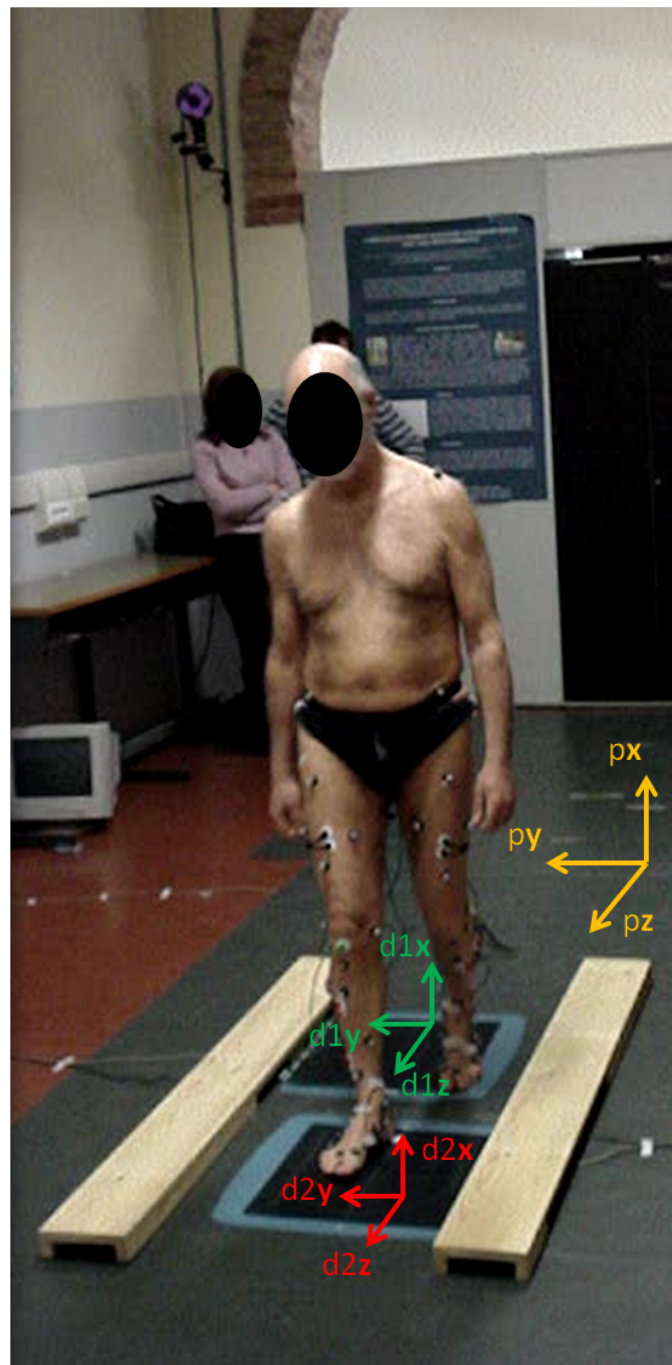
Figure 2.21: Example of a human movement analysis laboratory. Basic measurement instruments are depicted together with their systems of axes (p: photogrammetry; d: dynamometry). If level walking is analyzed, the motor task frame may coincide with the frame of one of the two force plates.
