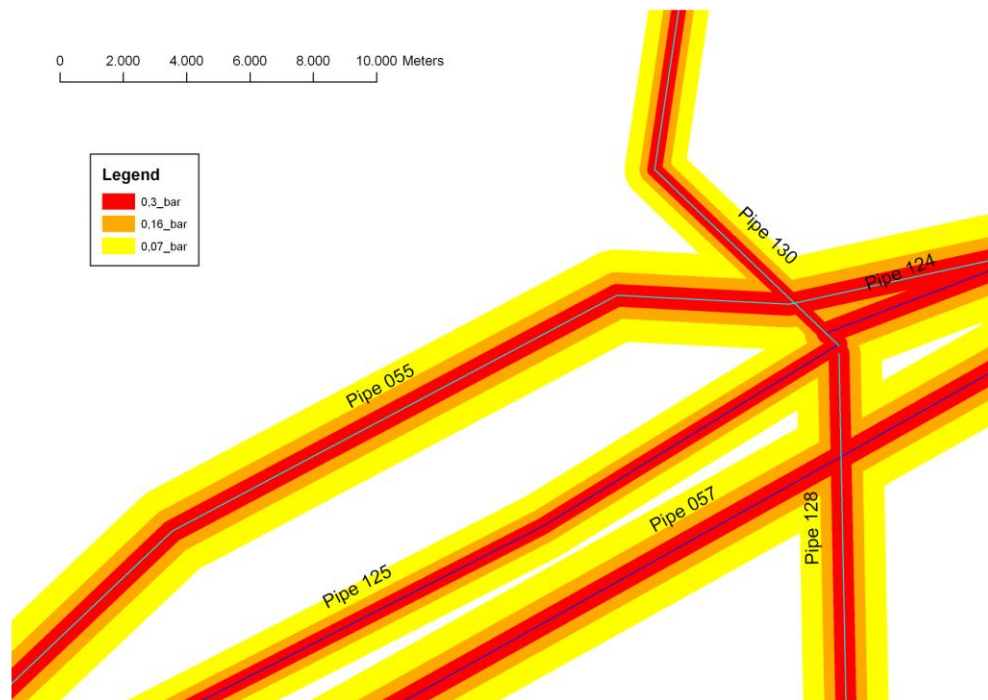
Figure 4.10 Vapour cloud explosion from horizontal release
