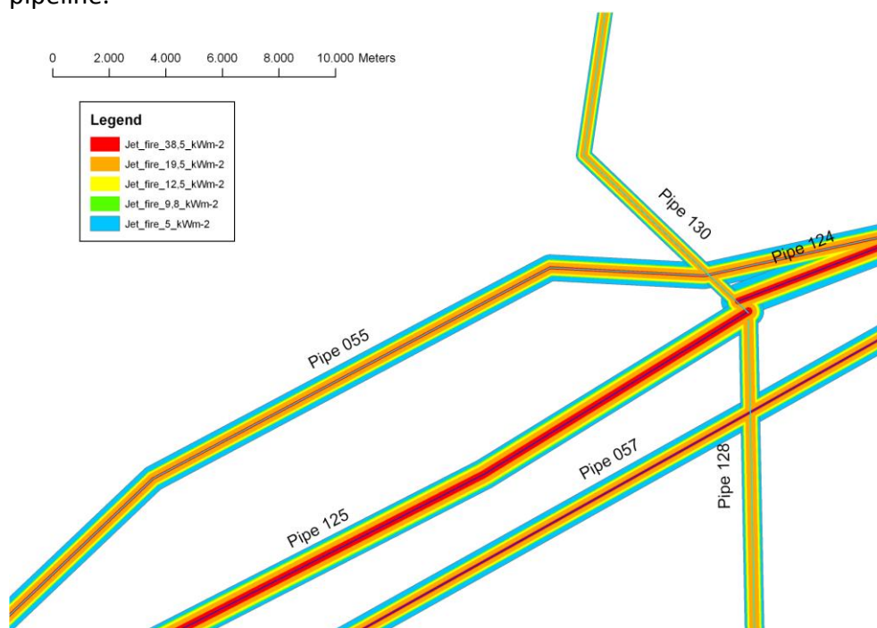
Figure 4.9 Jet fire from horizontal release
