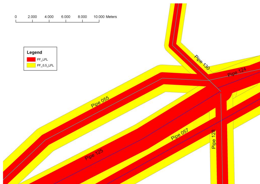
Figure 4.11 Flash fire from horizontal release
