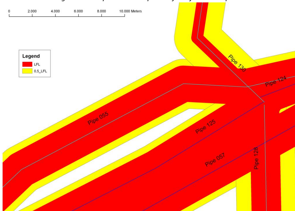
Figure 4.17 Flash fire from full bore rupture
