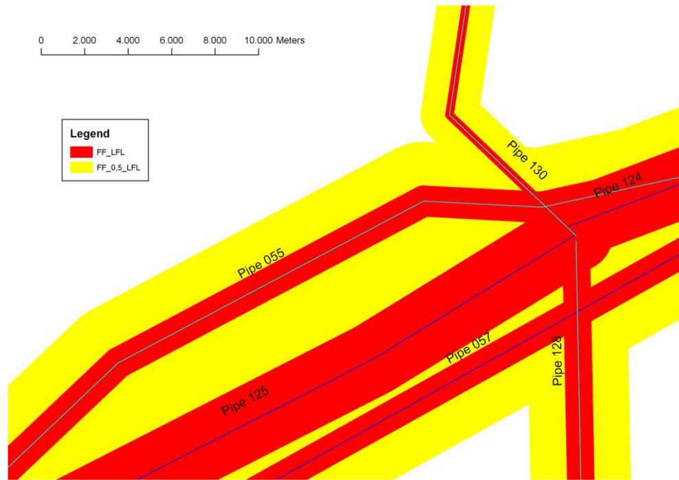
Figure 4.14 Flash fire from vertical release
