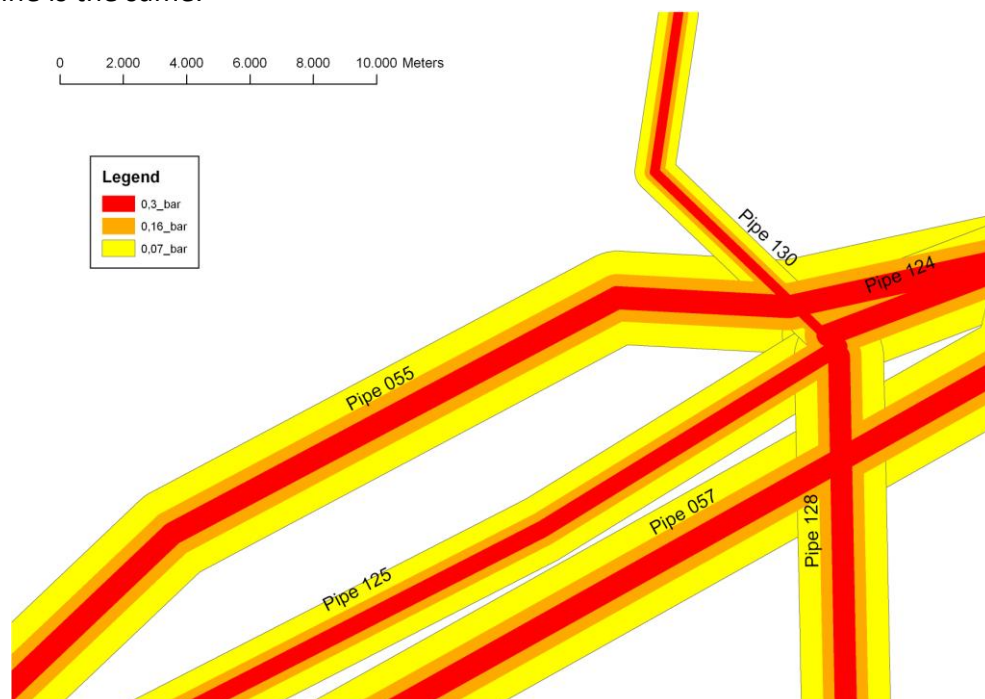
Figure 4.13 Vapour Cloud Explosion from vertical release
