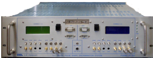
Figure 8.1: Front panel of a DPSD acquisition board.
