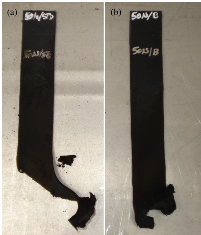
Fig. 5.10 Burned stripes of chloroprene-based compounds without (a) and with (b) glass powders.
