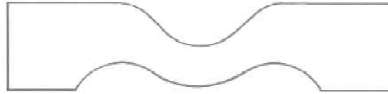
Fig. 4.14 Tear test piece.
