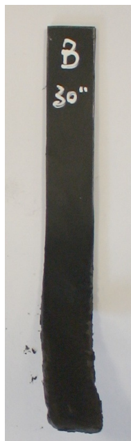
Fig. 5.6 Burned stripe of PF100-filled compound.
