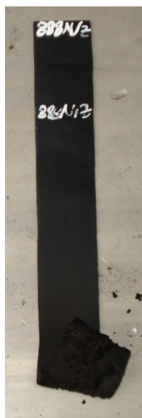
Fig. 5.8 Burned stripe of vulcanized compound.
