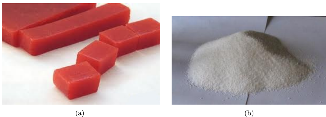
Figure 3.1: Examples of the two finished products: medicated jelly (a) and adsorbed-emulsion (b).
