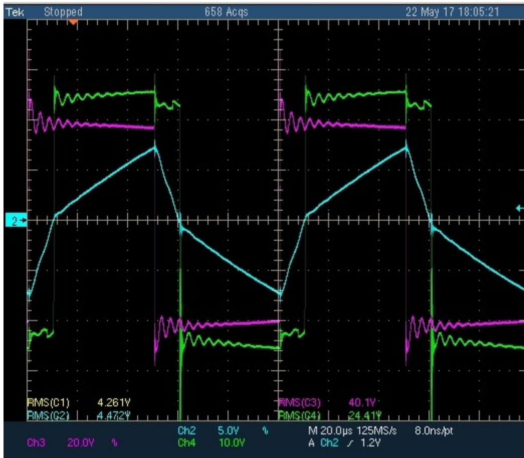
Fig.4.29 Voltage V_1 at the output of the input bridge (violet), voltage V_2 at the input of the output bridge (green) and inductance current(light blue).
