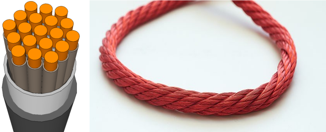
Fig. 2.15. Structure and example of Litz wire used in high frequency applications.
