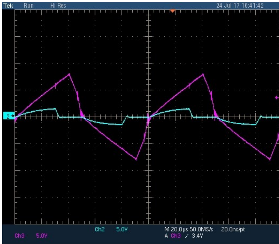
Fig. 5.40 Current at transformer side of port #1 (violet) and port #2 (light blue) referred to high voltage side.
