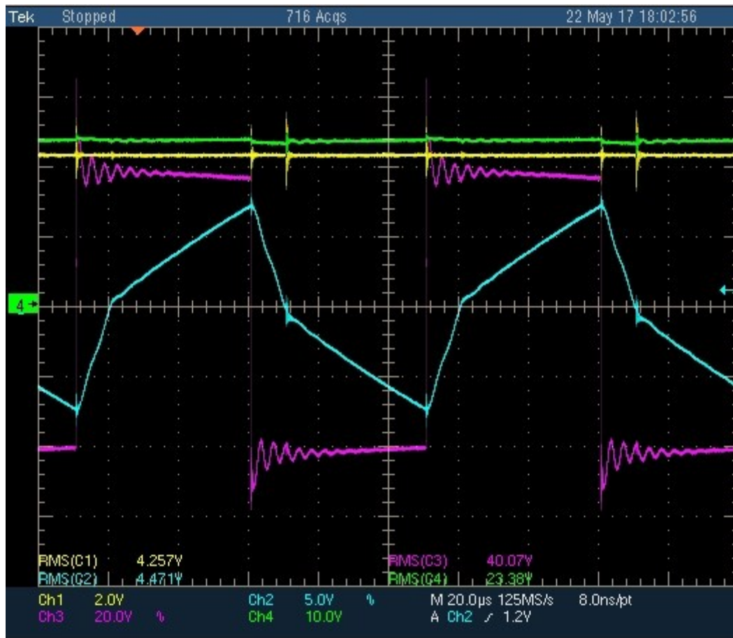
Fig.4.30 Output voltage (green) and current (yellow), voltage V_1 (violet) and inductance current (light blue).
