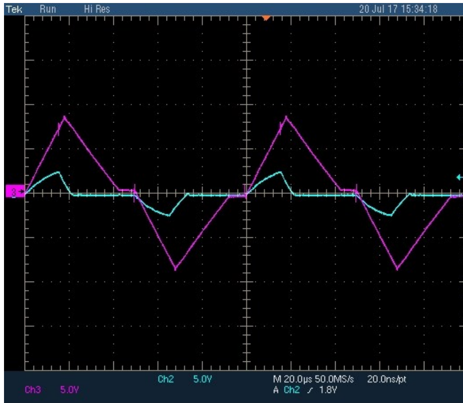
Fig. 5.34 Current at transformer side of port #1 (violet) and port #2 (light blue) referred at high voltage side.
