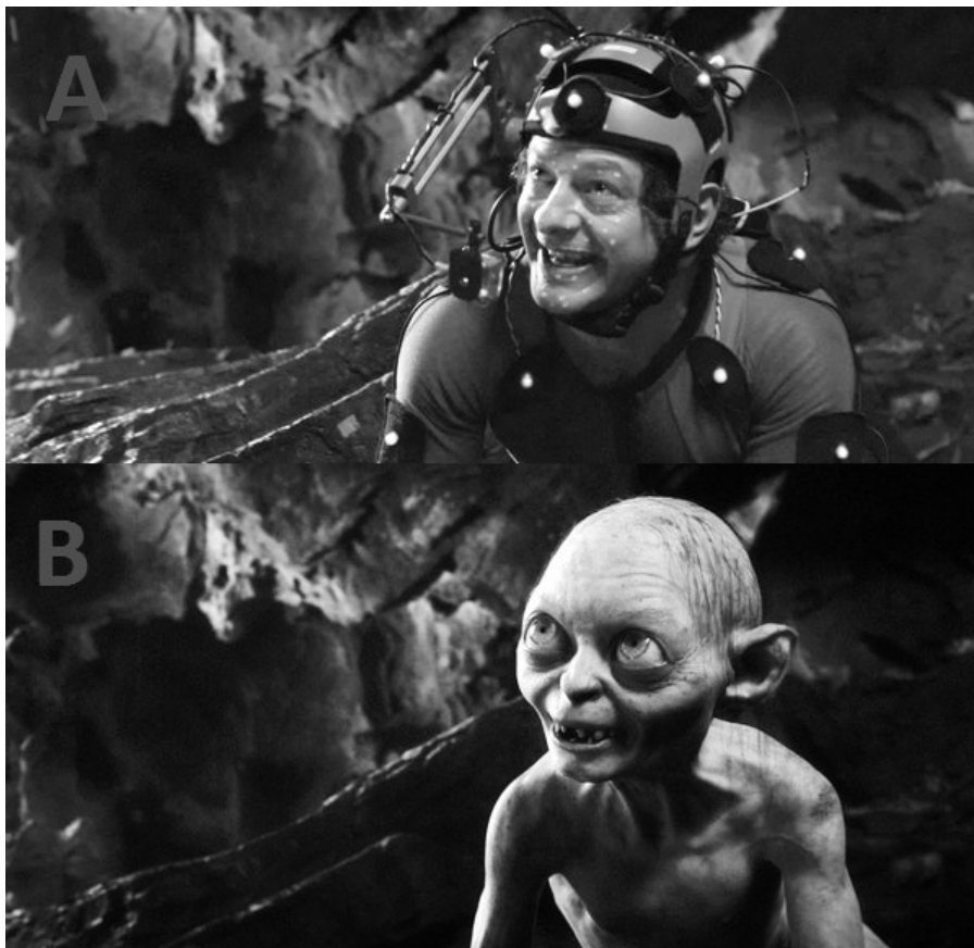
Figure 2. Motion capture technology developed from the need to use real acting to realistically animate digital characters. In panel A, a human actor is performing, the white dots on his head and body are markers used to extrapolate his tridimensional movement. In panel B the computed movements are assigned to a digital character.
