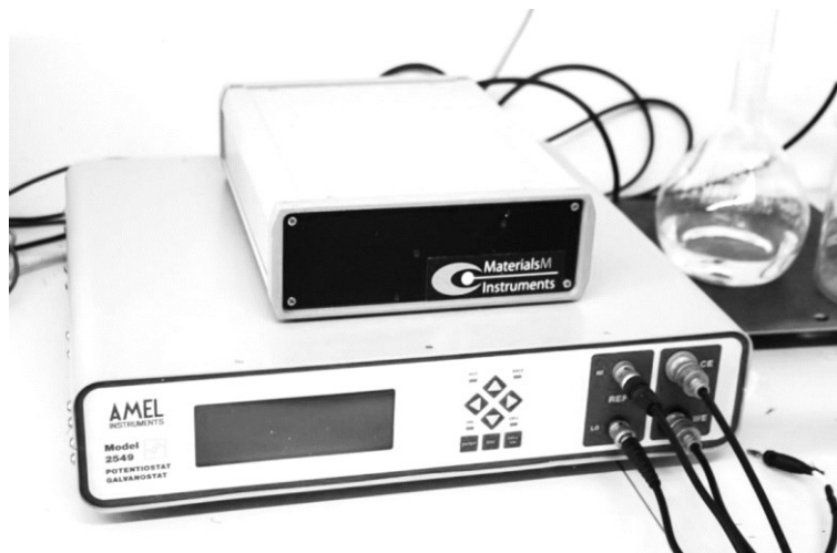
Figure 3.15 Potentiostat for the corrosion tests.
