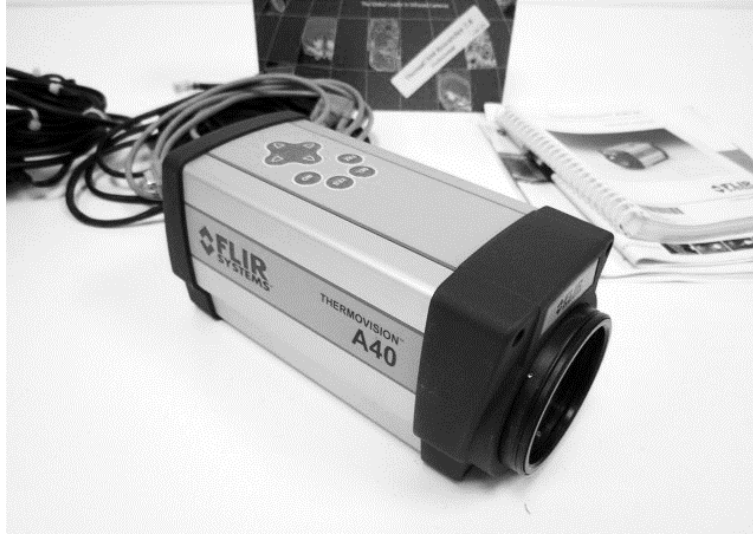
Figure 3.18 FLIR A40 Thermovision® thermal infrared camera.
