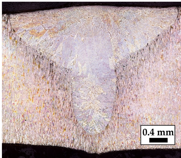
Figure 2 Overview of weld bead of the undeformed sample (electrolytic etching at 20 V with 20% NaOH).
