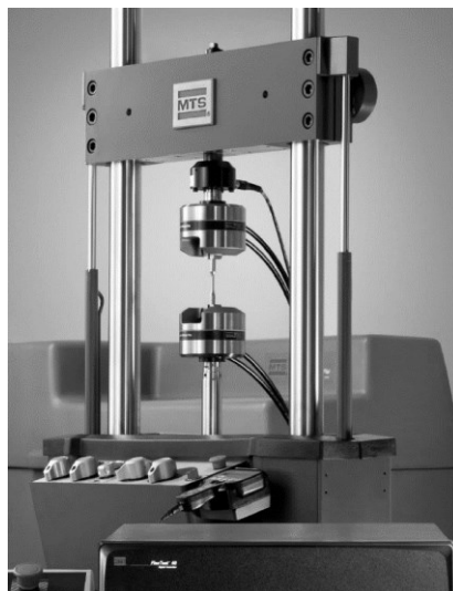
Figure 3.17 MTS 322 tensile test machine.
