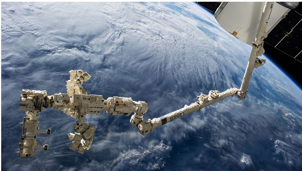
(b) SSRMS and DEXTRE attached to ISS with SpaceX Dragon cargo ship on the background
