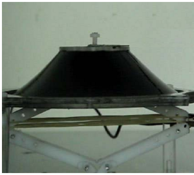
(a) Single-cone linear actuator with lozenge spring [73]
