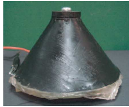
(b) Single-cone linear actuator with flexural springs (not visible) [74]
