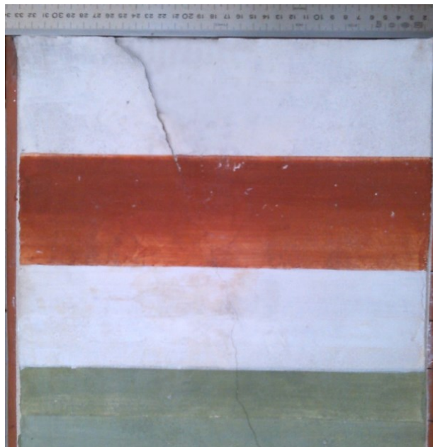
Figure 4.2: Fresco specimen, named “Stripe”, made with traditional techniques. The specimen width and height are equal respectively to 0.34 and 0.41 m.
