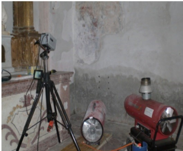
Figure 5.17: Experimental setup with the IR camera (on the left) and two air gun for forced ventilation (on the right).
