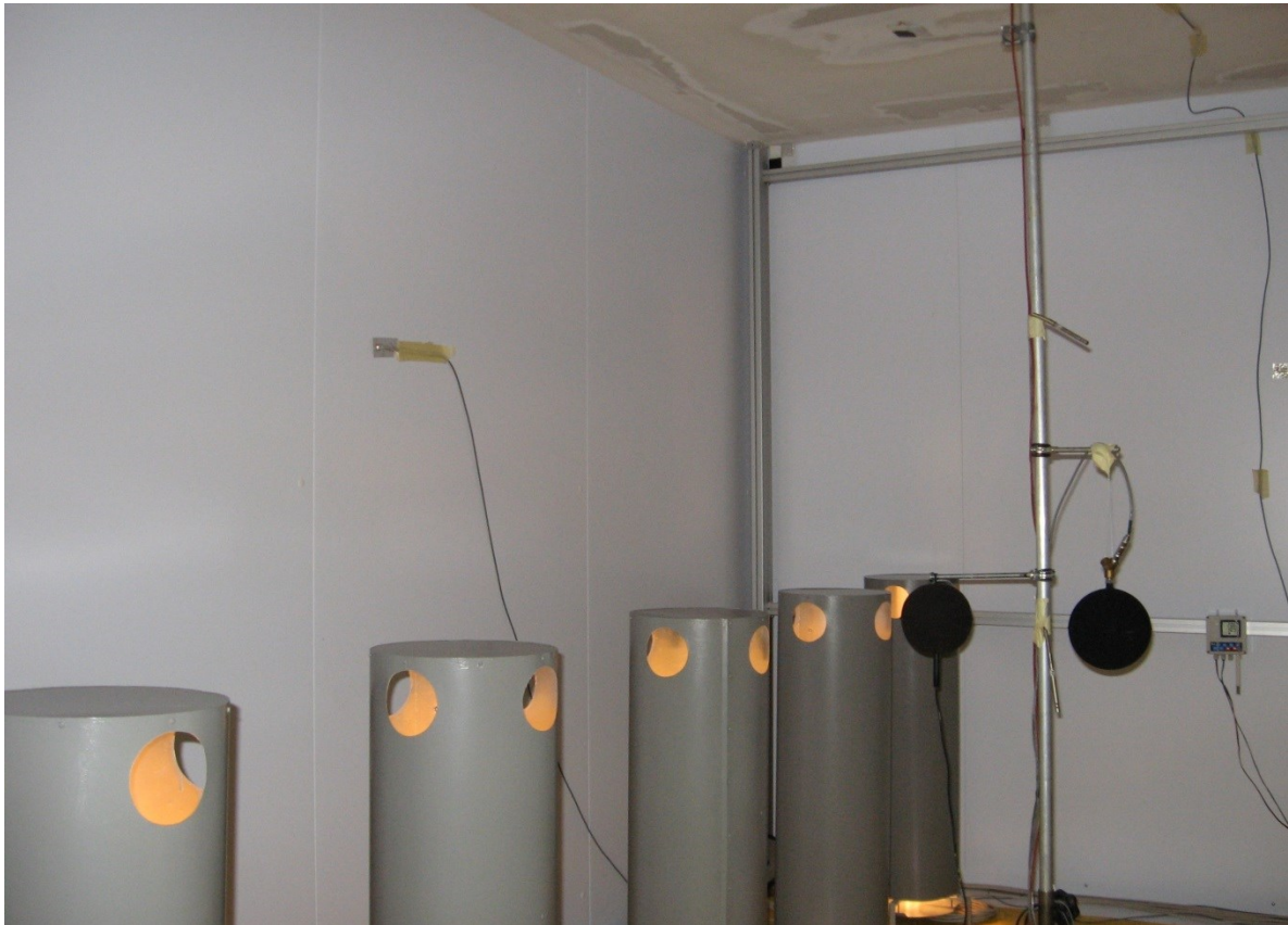
Figure 6.13: Thermal dummies inside the test room during the performance measurement of a radiant cooling system.
