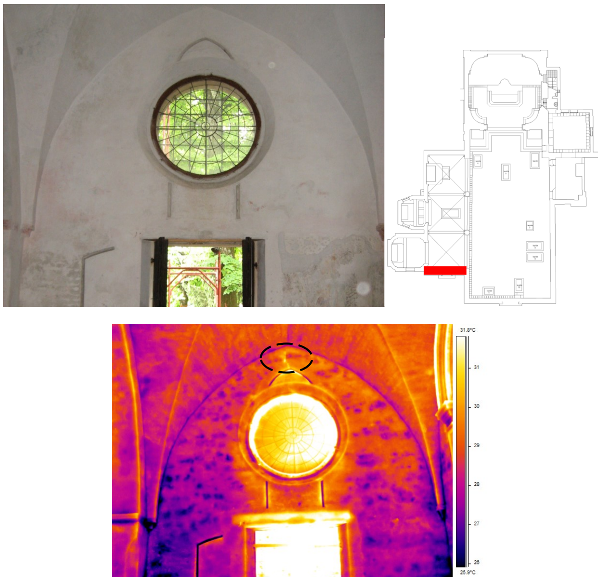
Figure 5.11: Photograph (left, top) of the investigated wall; air heaters are used as the thermal stimulus. Drawing (right, top) of the church, where the investigated wall is identified by the red rectangle. Thermal image (bottom) showing the wall structure and a small crack (black circle).
