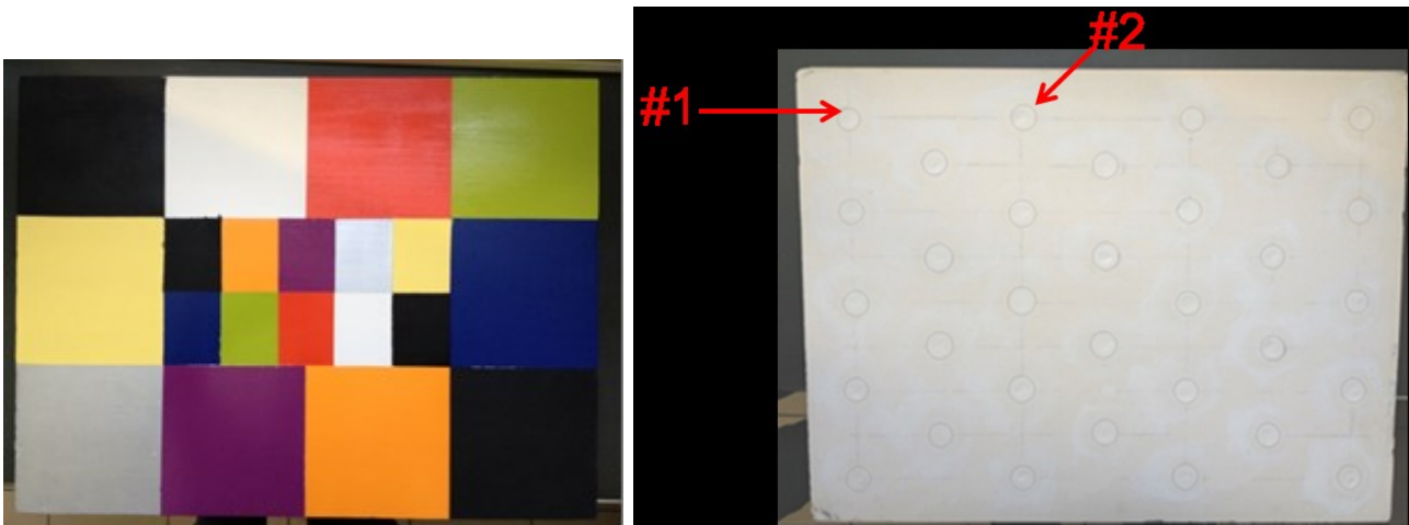
Figure 4.5: Fresco specimen, named “Squares”, painted with different colors (left image). Under the surface 32 circular defects were inserted (right image), two of them were named #1 and #2 respectively and taken as a reference.
