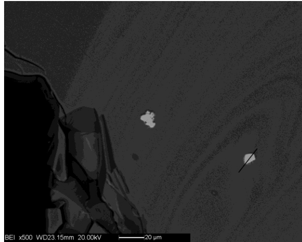
Figure 4.4.4: SEM-BSE image of normal section of sample ASO-20b. Dark grey area is blue glass of decorative rim. Two inclusions (paler grey) are embedded in glass matrix; black line: chemical profile shown in Figure 4.4.5.
