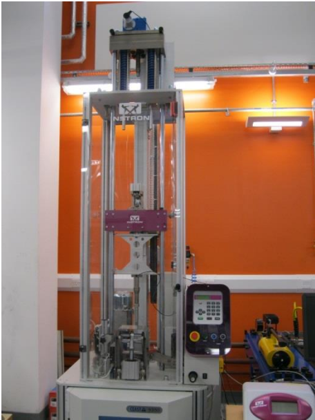
Figure 73: a) Plate and fixtures placed inside the drop tower chamber. b) Drop tower. c) Highlight on one PZT
