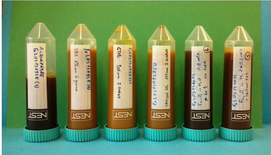
Figure 8.8: Fe_2O_3 water-based nanofluids prepared using single step method and different chemical agent to improve the stability.
