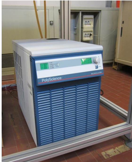
Figure 4.10: Cooling machine with turbine pump (Polyscience 5106T model).
