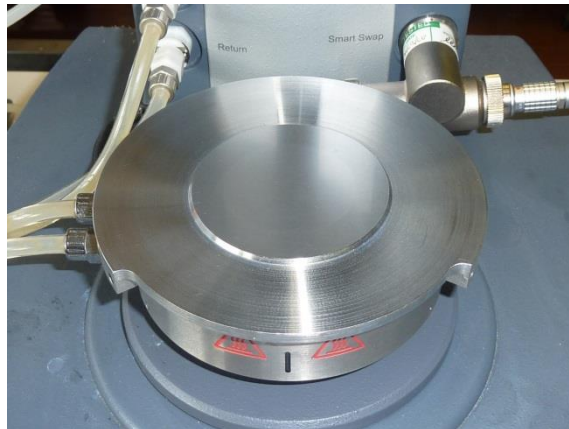
Figure 3.4: Peltier cover installed to homogenize the sample temperature.
