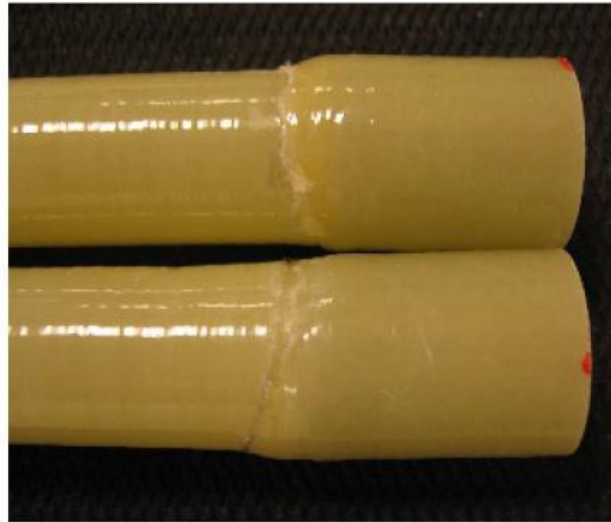
Figure 5: Defects near the end tabs
