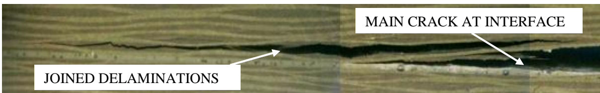
Figure 11: Joined delaminations and main crack interface propagation, mode mixity = 0.15
