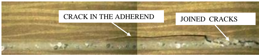
Figure 14: Joined inclined cracks and propagation in the adherend for mode mixity = 0.75
