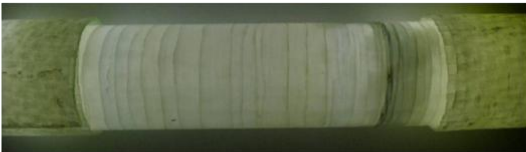
Figure 13: Multiple cracking in a [0_F/90_{U,3}] tube
