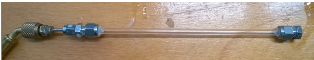
Figure 3.17. Glass tube for visualization during the leakages test.
