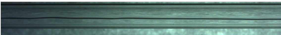
Figure 4.42. Flow pattern during condensation of R134a at 40°C saturation temperature, mass velocity equal to 50 kg m -2 s -1 and vapor quality of 0.45
