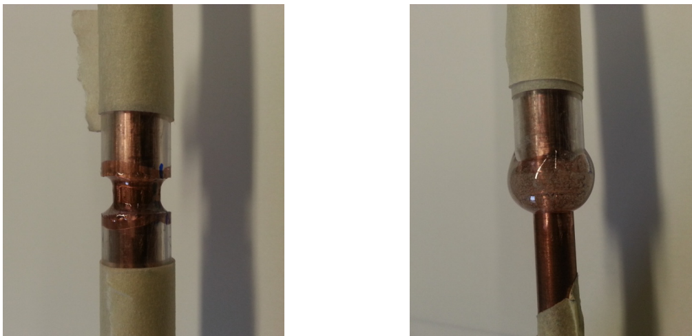
Figure 3.18. Gluing process of the lexan tubes and the copper tubes
