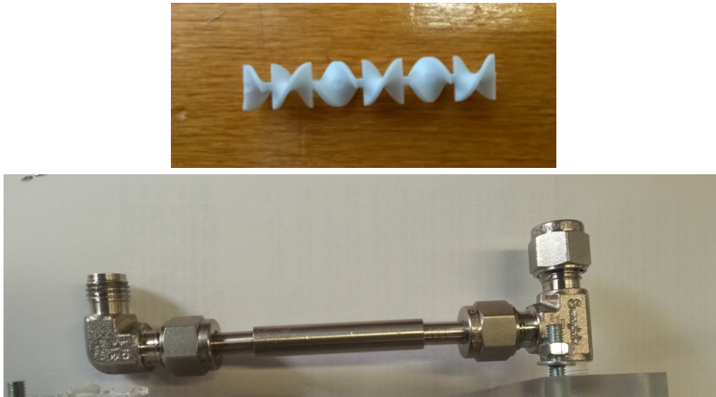
Figure 3.16. Mixer for the water side temperature measurements. Top: detail of the mixer. Bottom: stainless steel tubes for the connection of the mixer to the distributor and the temperature sensor
