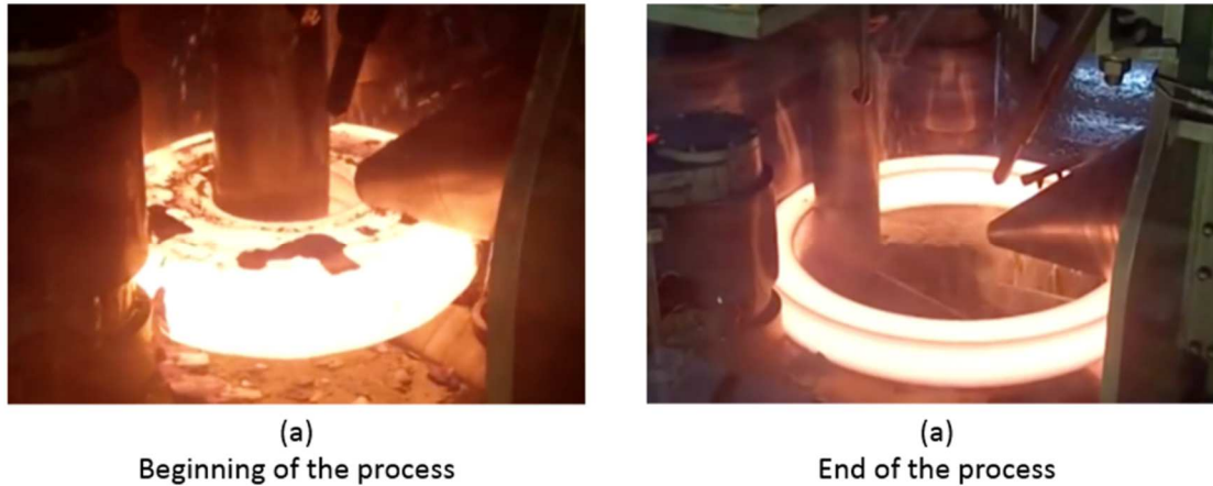
Fig. 2 – Ring blank at the beginning of the ring rolling process (a) and final ring at the end of it (b).
