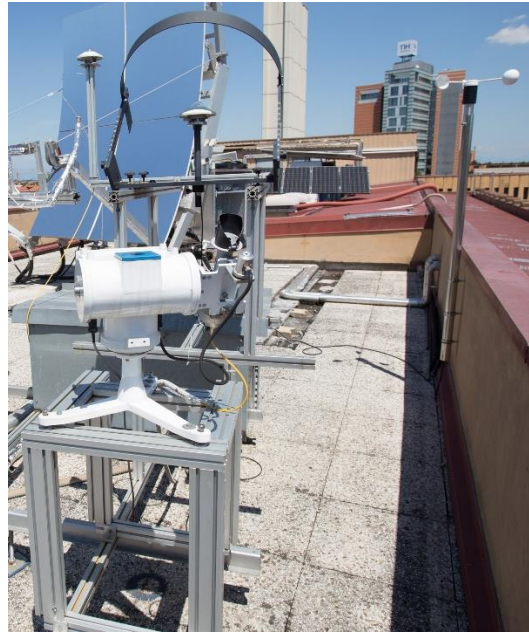
Figure 2 – Solar radiation measurement instrumentations installed on the roof of the Department of Industrial Engineering at the University of Padova.
