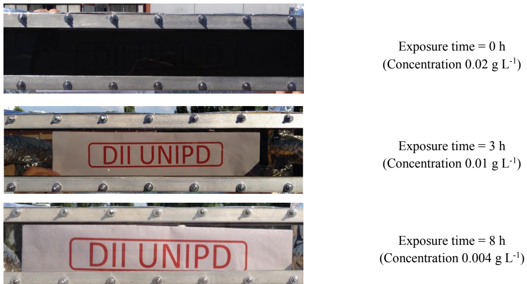
Figure 127 – Pictures of the nanofluid volume in the flow channel of the receiver taken at different exposure times.
