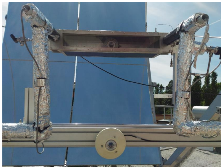
Figure 125 – Pyranometers for the measurement of the incoming solar radiation on the receiving plane and the transmitted solar radiation through the test section. The picture was taken before the circuit was filled with the nanofluid.
