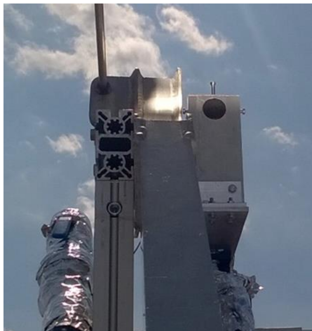
Figure 27 – Starting position of the heat flux microsensor. The electric linear actuator is completely down in its starting position, 65 mm under the ideal focal line of the concentrator.
