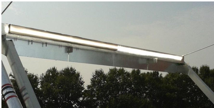
Figure 38 – Bar-and-plate flat receiver arranged on the support bar of the collector (a) and receiver under concentrated solar radiation during a test run (b).
