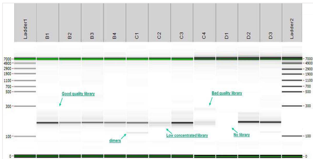
Figure 18: Pre-sequencing QC by Gel-electrophoresis. Representative gel of sncRNAs libraries shown good quality, presence of dimers, low concentration, bad quality or absence of fragments.
