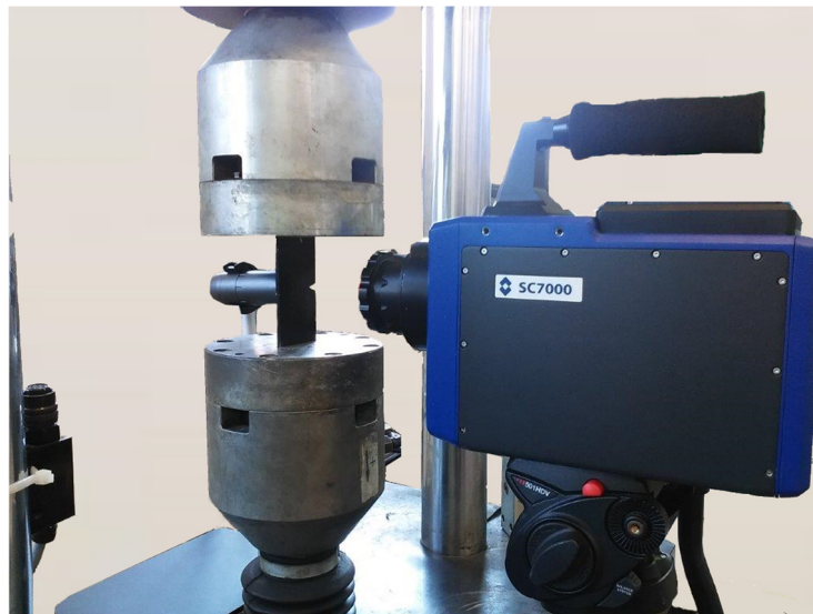
Figure 3.5: Test setup consisting of a FLIR SC7600 infrared camera, a AM4115ZT Dino-lite digital microscope and the specimen clamped in the test machine
