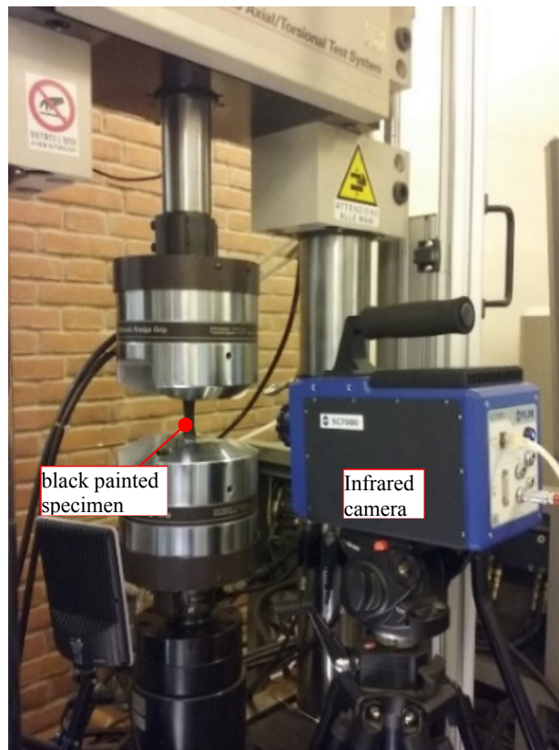
Figure 4.7: Picture of the experimental setup of multiaxial fatigue testing on type (B) specimens (Fig. 3b)
