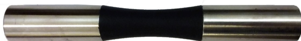
Figure 4.8. Picture of the specimens (B) of Fig. (3b), used for combined axial and torsional fatigue tests.
