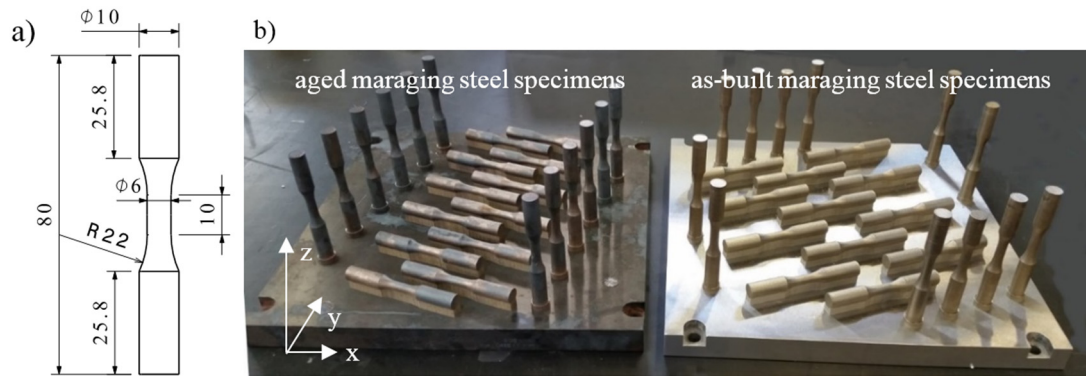
Figure 6.1: Specimen's geometry adopted for tensile static and fatigue tests on maraging steel produced by DMLS, and (b) two building platforms with the specimens produced by DMLS having specimen's axis oriented at 0^\circ and 90^\circ with respect to the building direction (z axis). [1]
