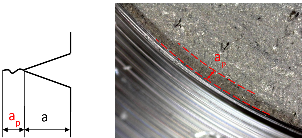
Figure 6.41: pre-crack a_p after fatigue failure.
