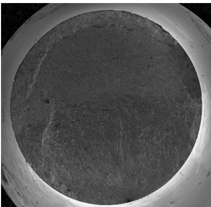
Figure 6.25: Examples of fracture surfaces relevant to the test series EN_0°_T and relevant \sqrt{\text{area}} at the failure origin.
