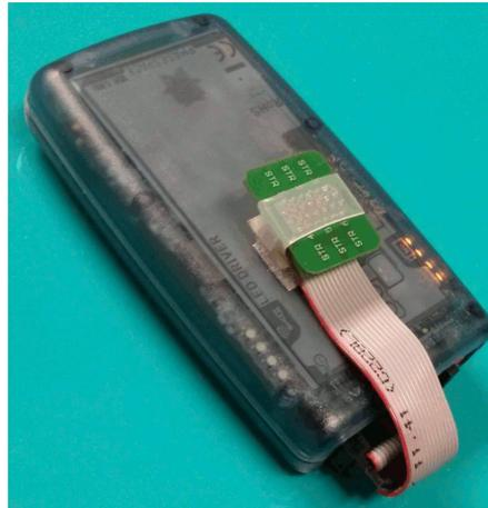
Figure 4.9: The LED driver unit communicates with the base station and can drive up to 72 active markers.
