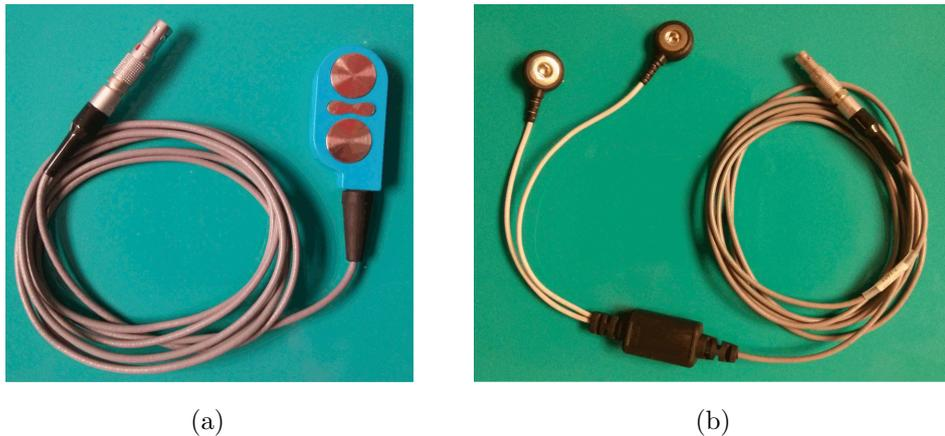
Figure 4.4: (a) Dry electrode considered in a preliminary stage. Due to the high rigidity of the housing they were not suited to collect data of shoulder muscles. (b) MA-420 differential input probe, with snap contacts and preamplifier. This probe can be used with the Norotrode 20 disposable electrodes.
