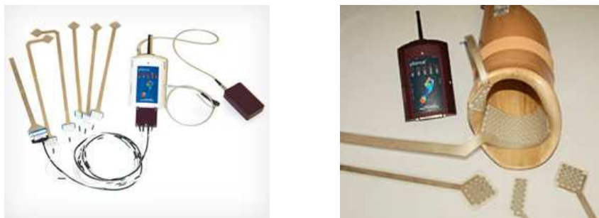
Figure 7.1 - Novel Prosthesis System: Pliance-RLS system, RLS sensors with different standard shapes.
