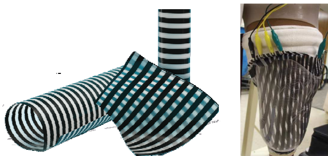
Figure 7.2 - Zebra™ 3D System: Zebra sheet sensors and thermoformed sensors within the prosthetic socket.
