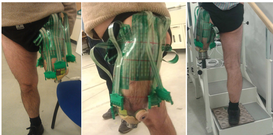
Figure 7.6 – Patient wearing the instrumented socket (left and middle) and patient with the prosthetic socket positioned on the trestle for the acquisition phase (right).
