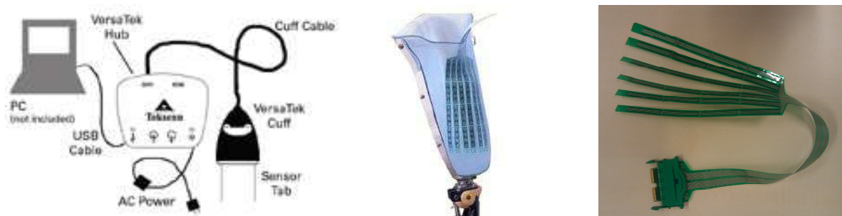
Figure 7.3 - F-Socket Pressure System: scanning electronics (left), software (middle) and patented thin-film sensors (right).
