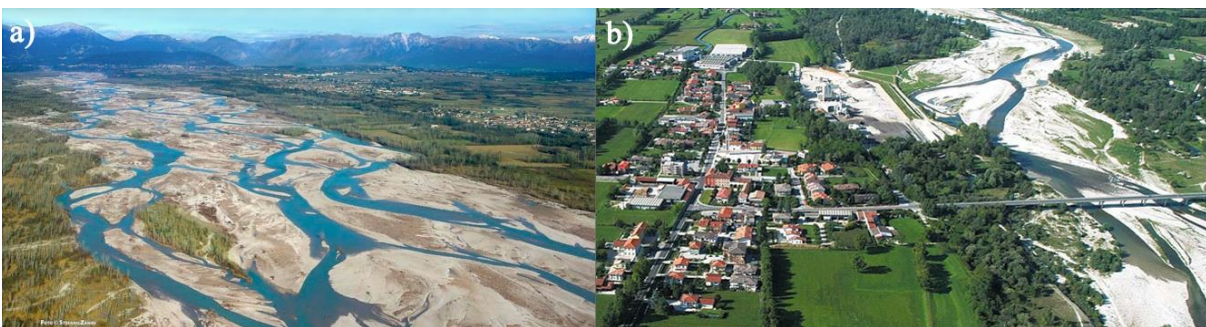
Figure 6. Typical braided reach (a) of the Tagliamento River (Italy) and typical wandering reach (b) of the Brenta River (Italy).
