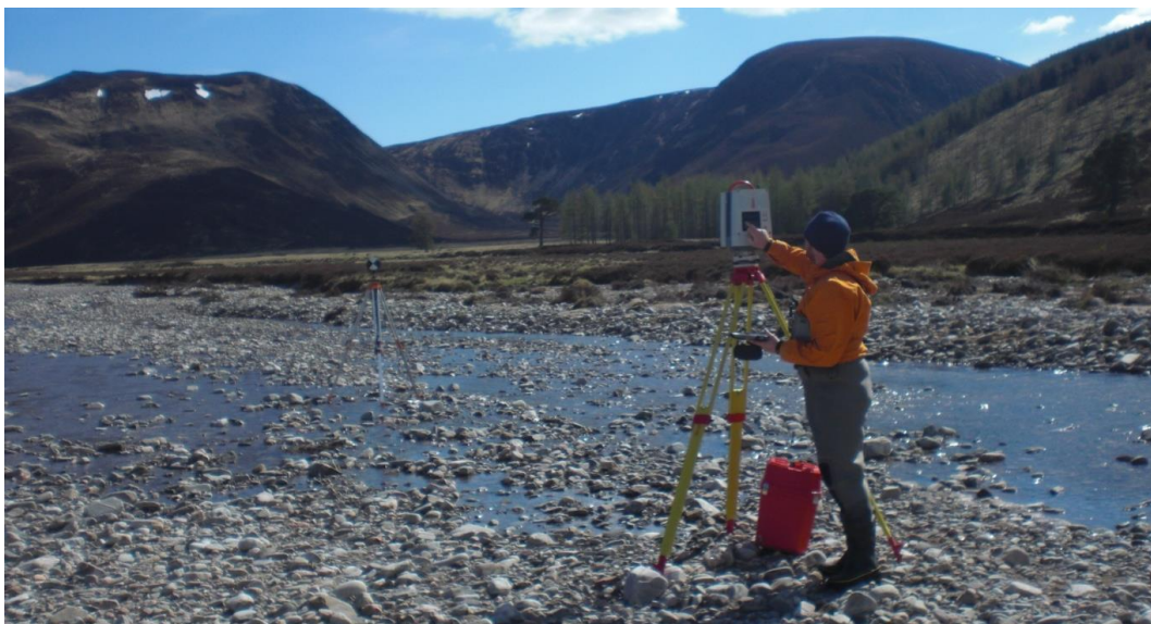
Figure 17. Field data acquisition with Terrestrial Laser Scanner on Feshie River (Scotland).
