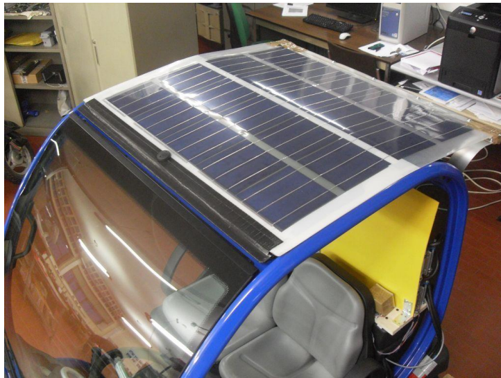
Fig.7.7.1 mini-electric car Birò Estrimà with implanted 20 Cell SilFab PV panel
