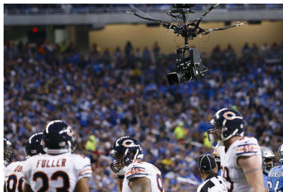
Figure 1.3: Cable Camera in action during a football field
