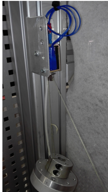
Figure 7.5: Third cable connected to the electromagnet
