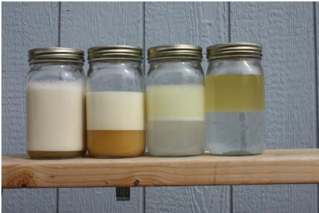
Figure 2. In sequence from left to right, different steps of the collapse of an oil-in-water emulsion. On the left, freshly prepared emulsion; on the right, complete separation of the phases.
