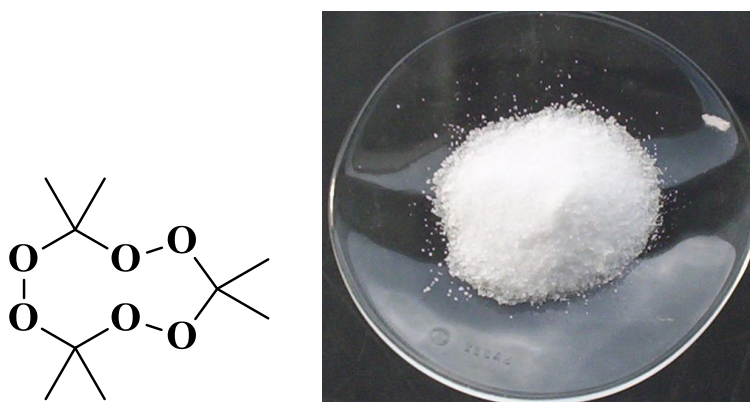
Figure 10. On the left, chemical structure of triacetone triperoxide and, on the right, the appearance of its solid form.
