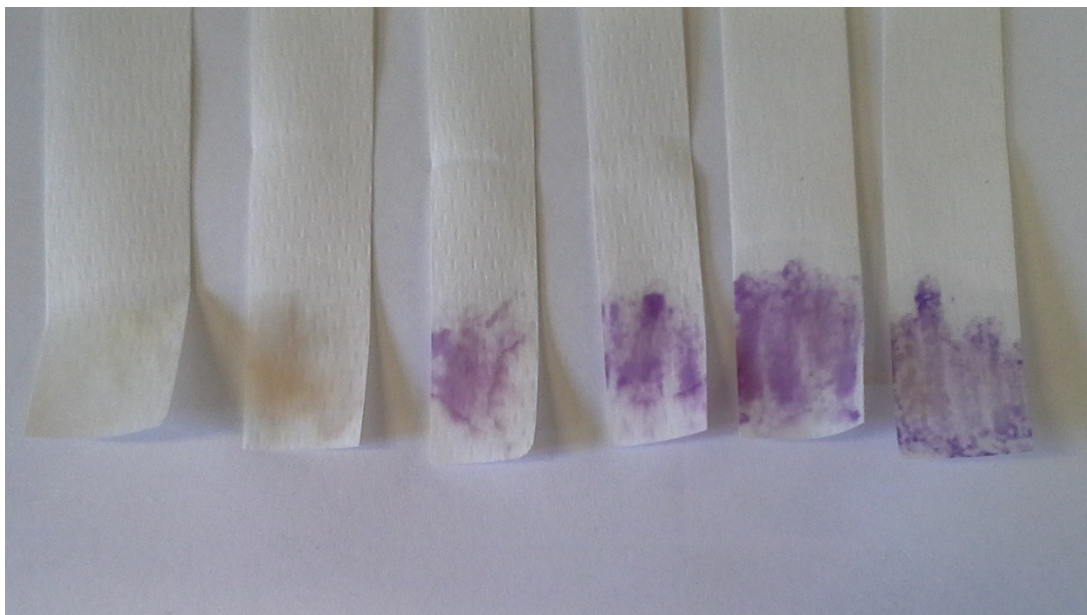
Figure 29. Paper strips used for the test on (from left to right) pure water, 0.1%, 0.5%, 1%, 5%, 10% solutions of acetone.
