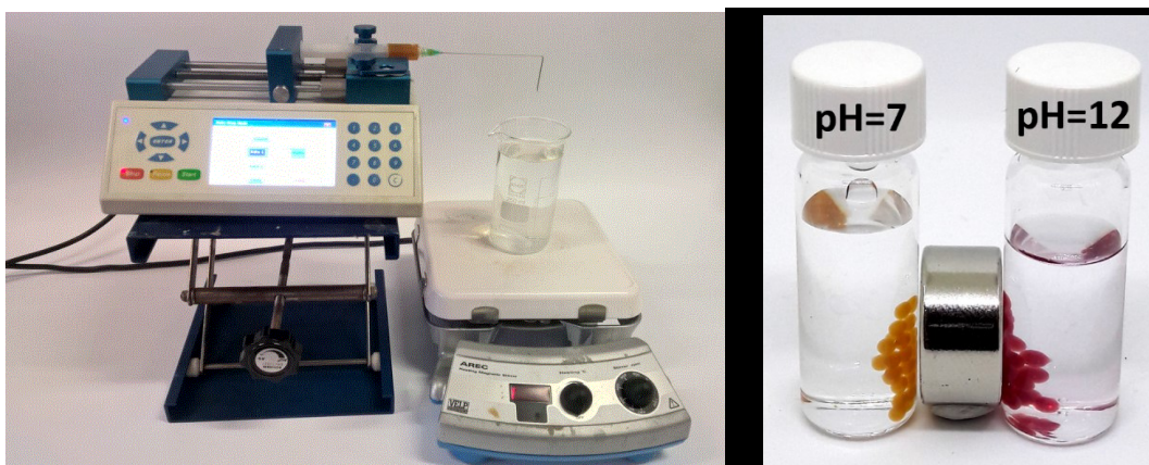
Figure 61. On the left, the device used for the preparation of the beads (syringe pump, syringe with alginate, becker with \text{CaCl}_{2(aq)} ). On the right, example of double stimuli-response of the beads to pH variation and magnetic stimulus.
