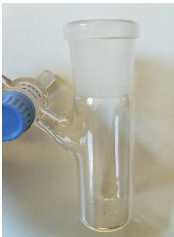
Figure 24. Image of the reactor for photocatalytic oxidations.
