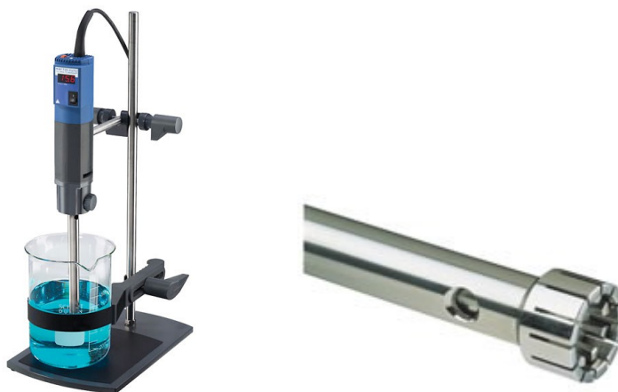
Figure 14. On the left, picture of the homogenizer. On the right, particular of the rotor-stator equipment.
