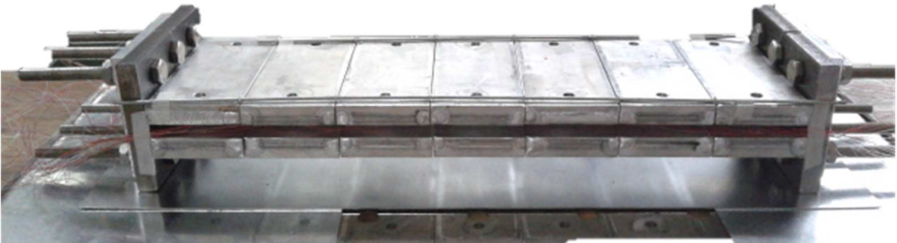
Figure 2.9. Test section with water module bonded after 2h at 150 °C.
