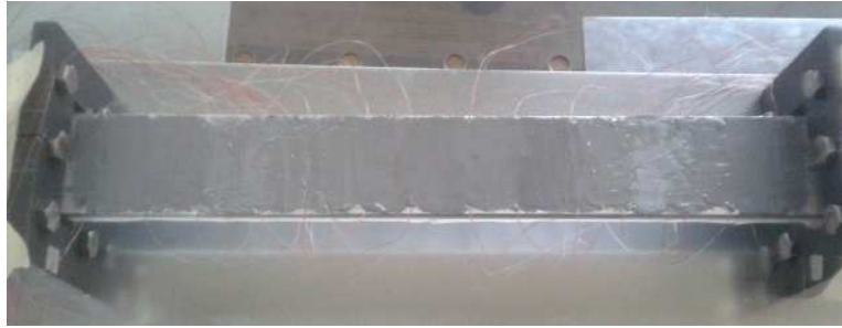
Figure 2.8. Test section with aluminium based conductive paste before the attachment of water modules.
