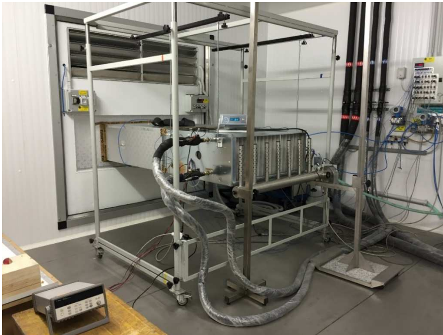
Figure 1.1. Experimental set up: climatic chamber with the tested machine connected to the aeraulic tunnel through a plenum.
