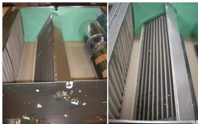
Figure 1.17. Photos of experimental test section with the finned tube heat exchanger with two different tilt angles.
