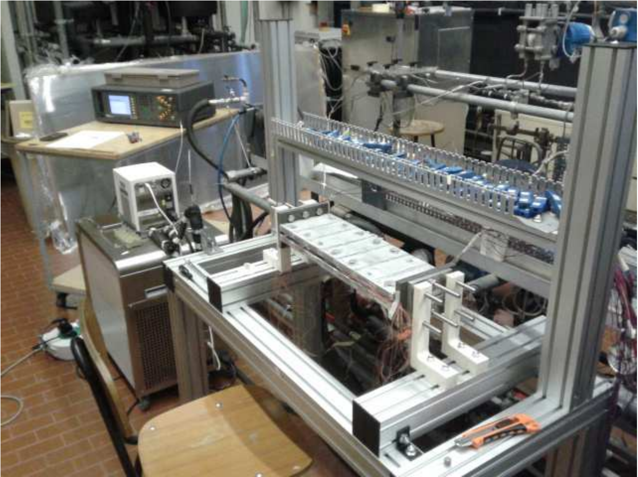
Figure 2.11. Test section and instrumentation used for on site calibration of the 56 thermocouples.
