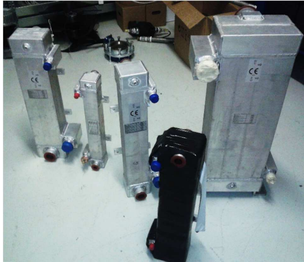
Figure 5.2. Bar and plate heat exchangers with different sizes that have been tested in direct expansion systems.
