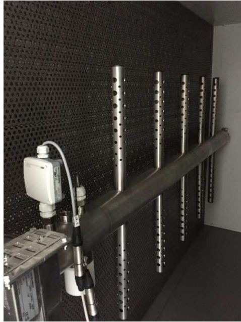
Figure 1.2. Air sampling tube for the measurement of temperature and humidity of air in the aerodynamic tunnel.
