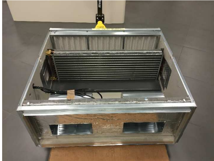
Figure 1.4. Tested machine (EBH 020-3R) with three rows heat exchanger.
