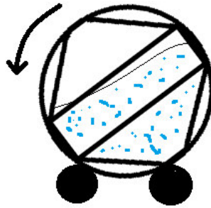
FIGURE 4.5: A picture of the cylinder containing the double cone placed on two rollers.
