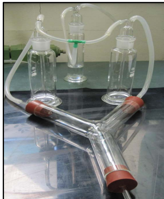
Figure 2- The vertical glass Y-olfactometer used in the experiments
