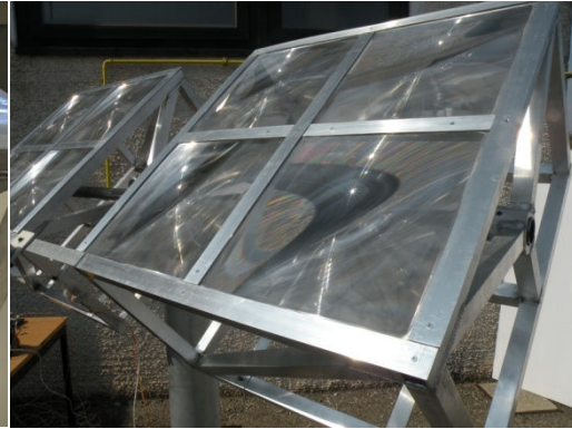
Figure 5.6. Solar collector: frames integration.
