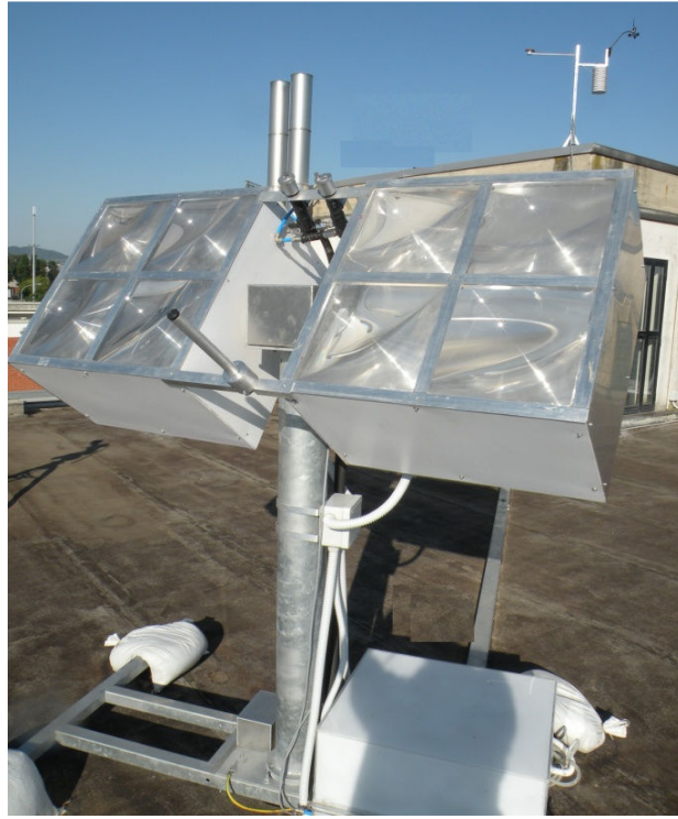
Figure 5.1. Concentrating PV/T prototype, front view.
