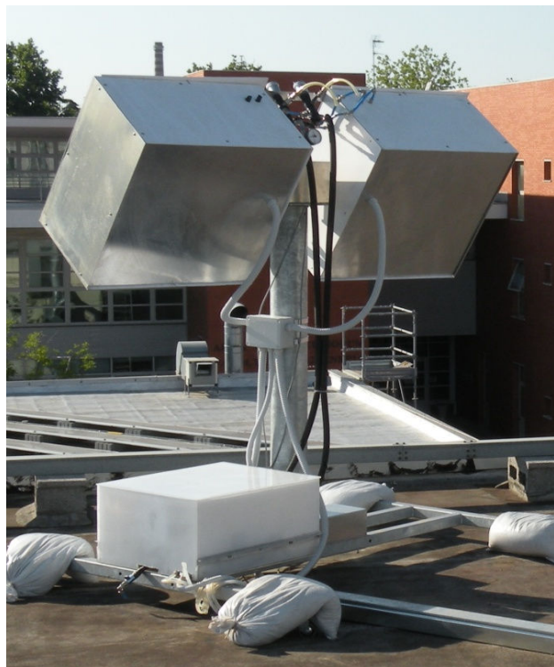
Figure 5.2. Concentrating PV/T prototype, back view.
