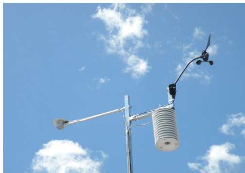
Figure 5.24. Weather station integrating the pyranometer, the air temperature thermometer and the anemometer.
