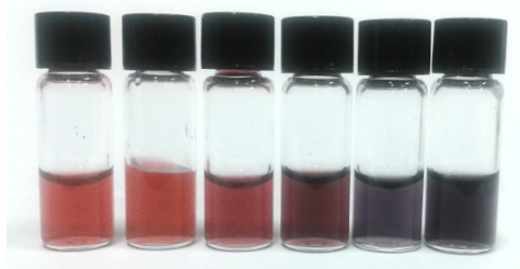
Figure 5.8: Au NPs solution at different probe molecular concentrations, rising from left to right.
