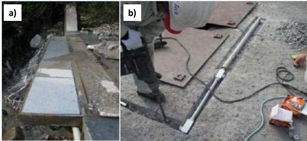
Figure 13: Swiss (a) and Japanese (b) geophones.
