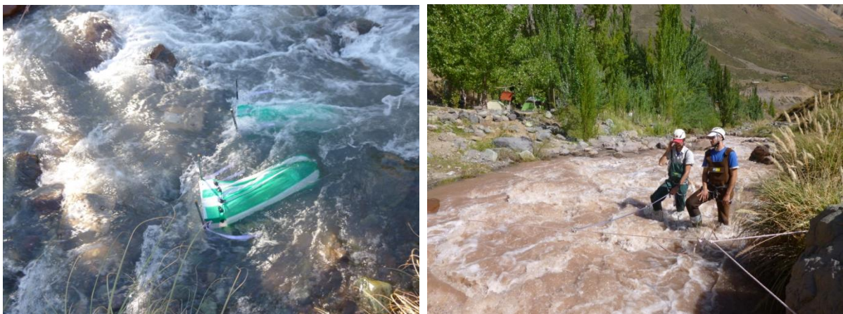
Figure 11: Bunte sampler in Estero Morales (on the left), and phase of retreat of the samplers (on the right).
