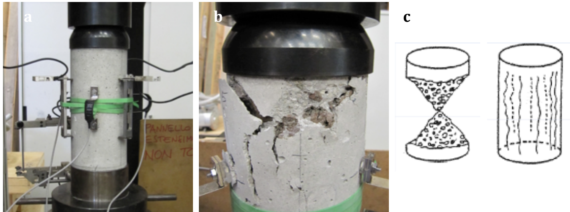
Fig. 11 – a) Experimental set up for the determination of the elastic modulus and compressive strength. b) Failure of a LWAC sample in compression. c) Satisfactory failures of standard specimens according to EN 12390.
