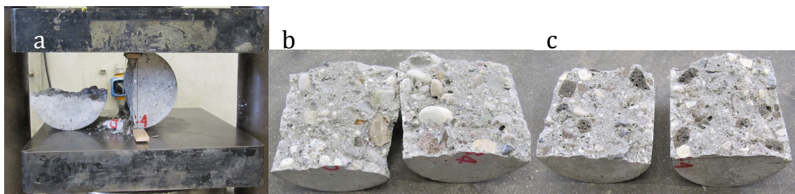
Fig. 12 – a) Brazilian test set up. b) Failure of a sample using traditional aggregates. c) Failure of a LWAC sample.
