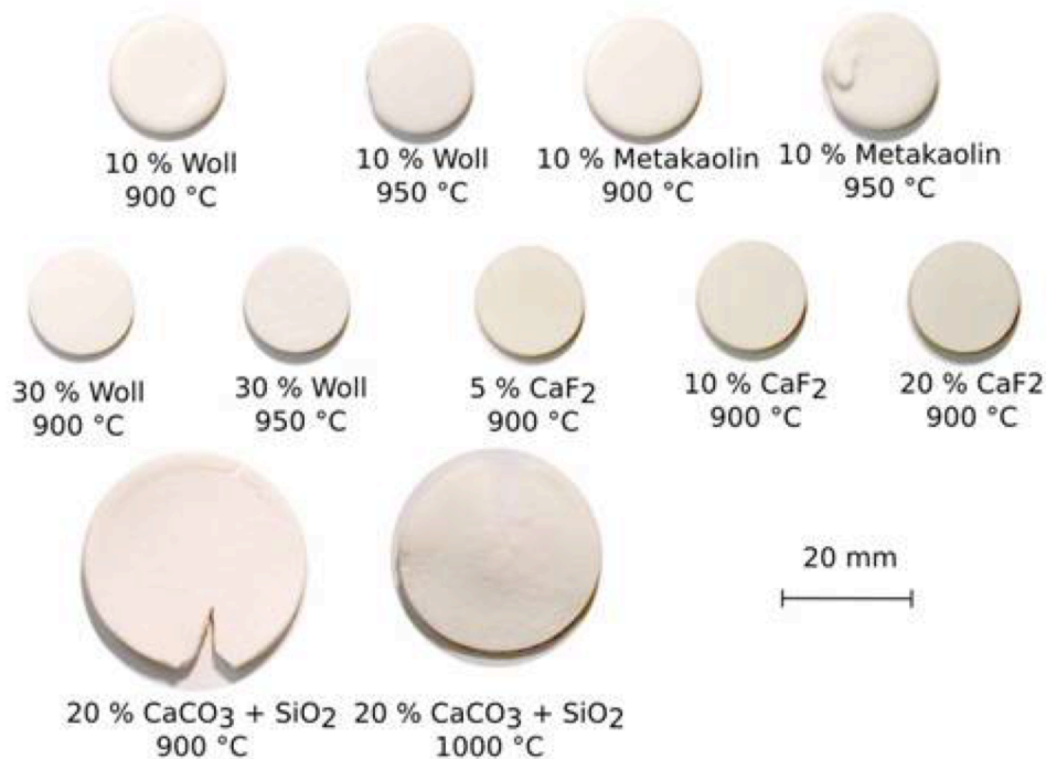
Fig. 29 – White glass ceramics composed prevalently of cullet 95 -70 wt% and a whitening agen. The samples of larger diameter (20% CaCO 3 + SiO 2 ) were pressed in a mould with Ø=31 mm.
