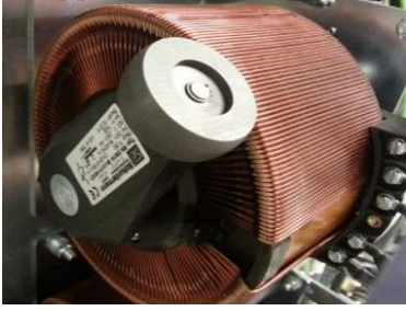
Figure 2.23: Single-phase toroidal transformer with continuous tap selector.
