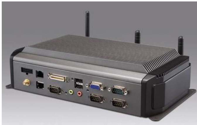
Fig. 6.15 The Advantech TREK 550 automotive PC
