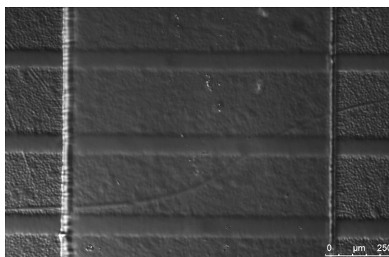
Figure 2.3.9 Linear pattern of polyacrylamide formed across a stretching chamber of the microfluidic stretching device. The pattern forces cells to align parallel to the main direction of deformation.
