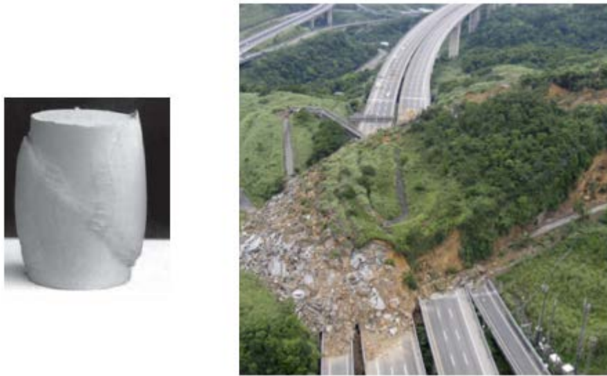
Figure 1.1: Strain Localization: experimental evidence [12] and real massive landslide obstructing highway in Taiwan.
