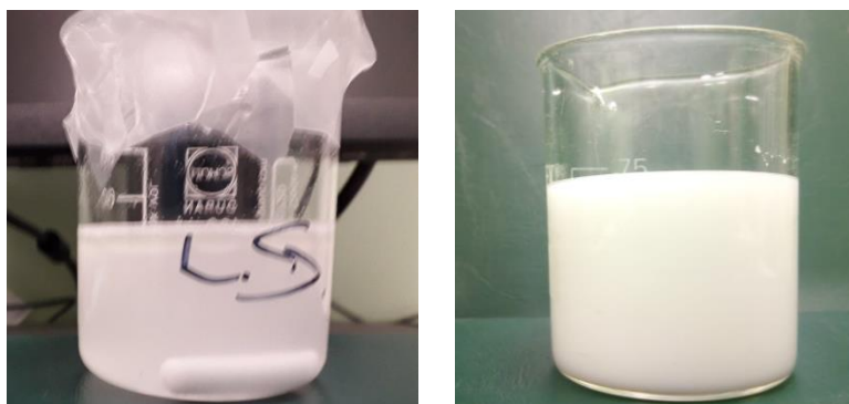
Figure 7.2. Emulsions with ammonium lauryl sulfate (left) and Span 80 / Tween 80 (right)
