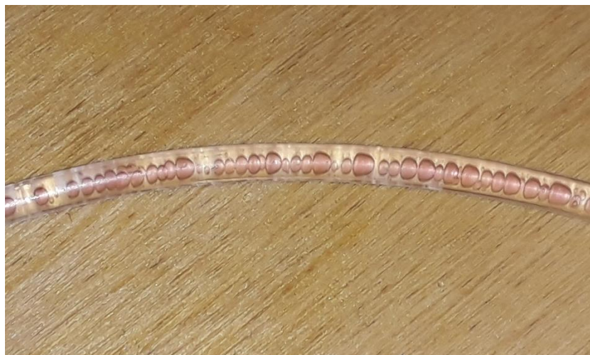
Figure 7.1. Biphasic stream of water droplets in oil.
