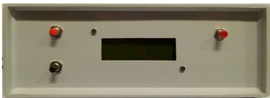
Figure 2.6. Power controlled power supply for the calibration of the calorimetric reactor.
