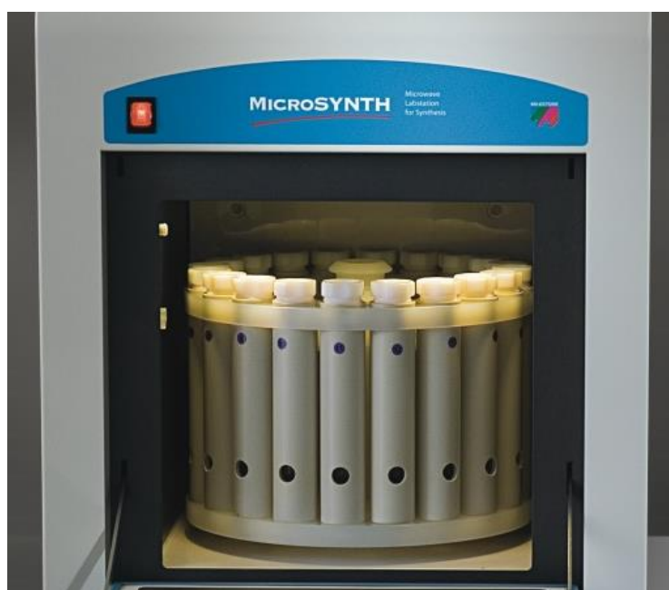
Figure 2.8. Microsynth microwave reactor [1].
