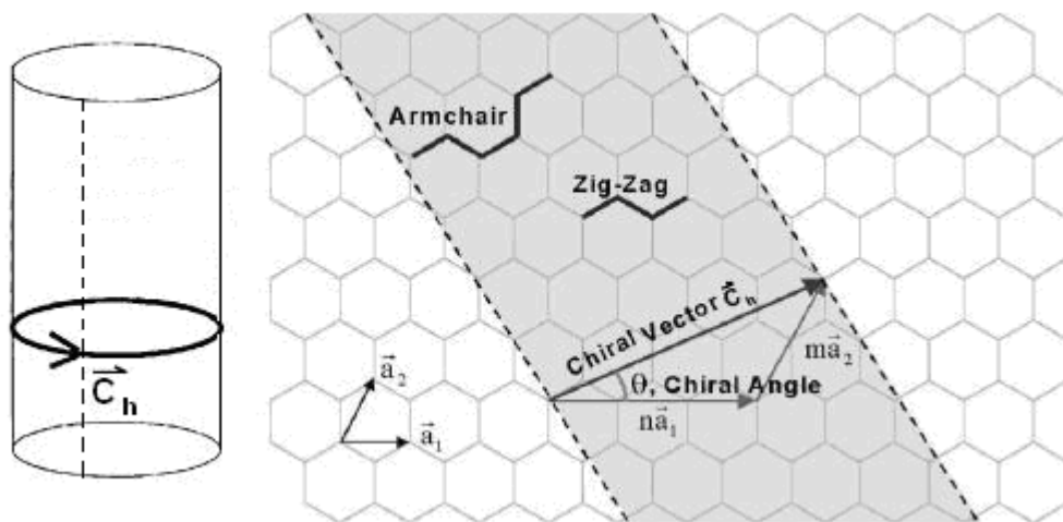
Figure 1.26. The chiral vector and the chiral angle in a carbon nanotube (Thostenson et al., 2001; Cohen, 2001; Thostenson et al., 2005).
