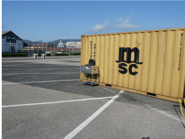
Figure 7.2: SMANDRA determines the position of the radioactive source inside the container
