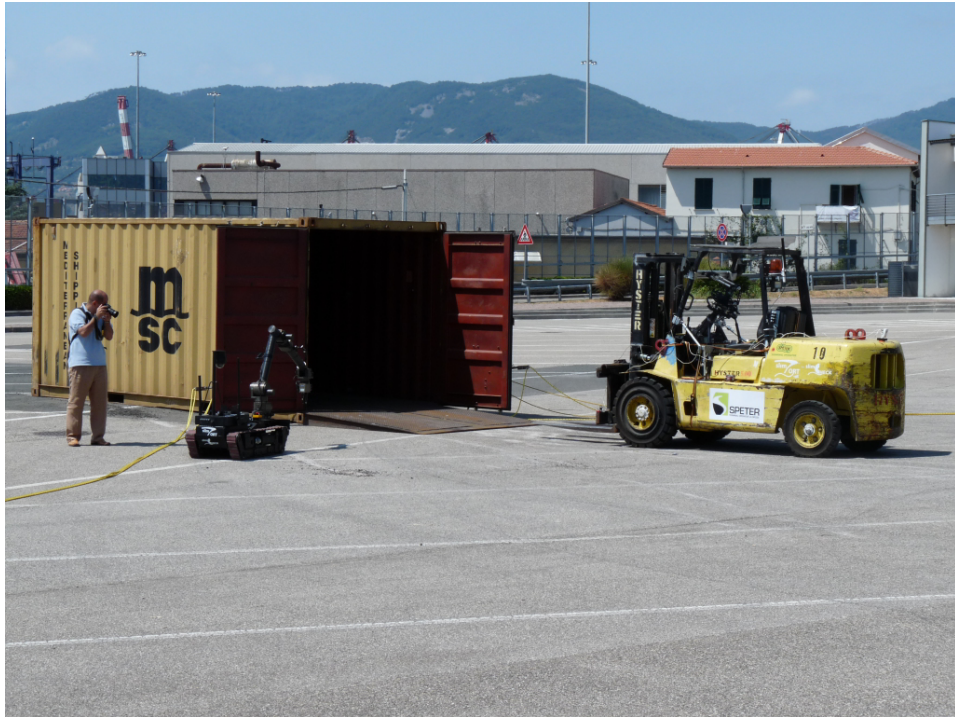
Figure 7.4: The remote controlled robotic arm entered the container after removals of pallets
