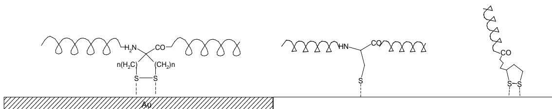
Figure 3. Comparison between different linkage models. Adt linkage (on the left) should be more rigid than cysteine one (in the middle) and permit a closer placing of peptides than lipoic acid linkage (on the right).
