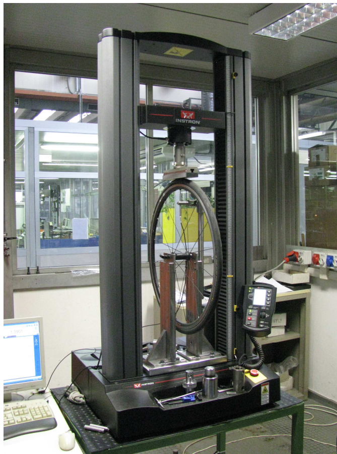
Fig. 4.27 Test bench developed for static radial test.
