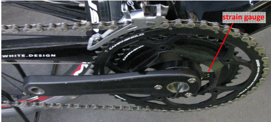
Fig. 17.4 Spider arm of the crankset instrumented with strain gauges.
