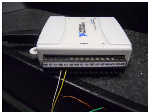
Fig. 4.30 NI USB-6008 data acquisition system.
