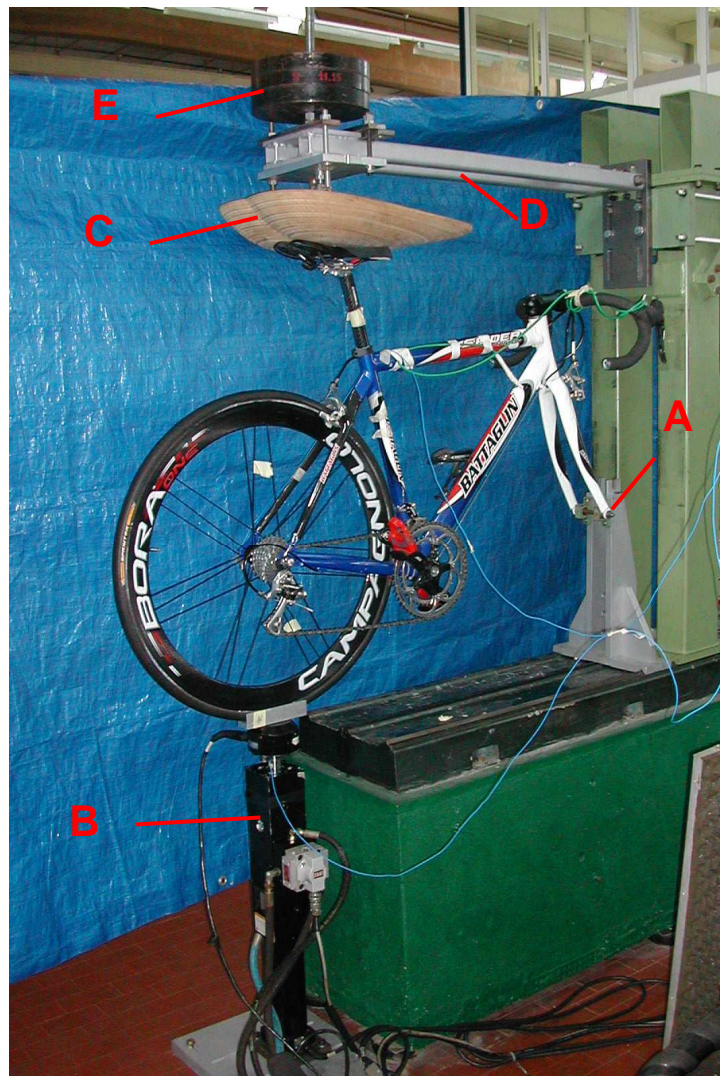
Fig.5.3 Test bench. A: front fork axle hinge; B: servohydraulic cylinder; C: wooden dummy bottom; D: swinging beam; E: dead weights.
