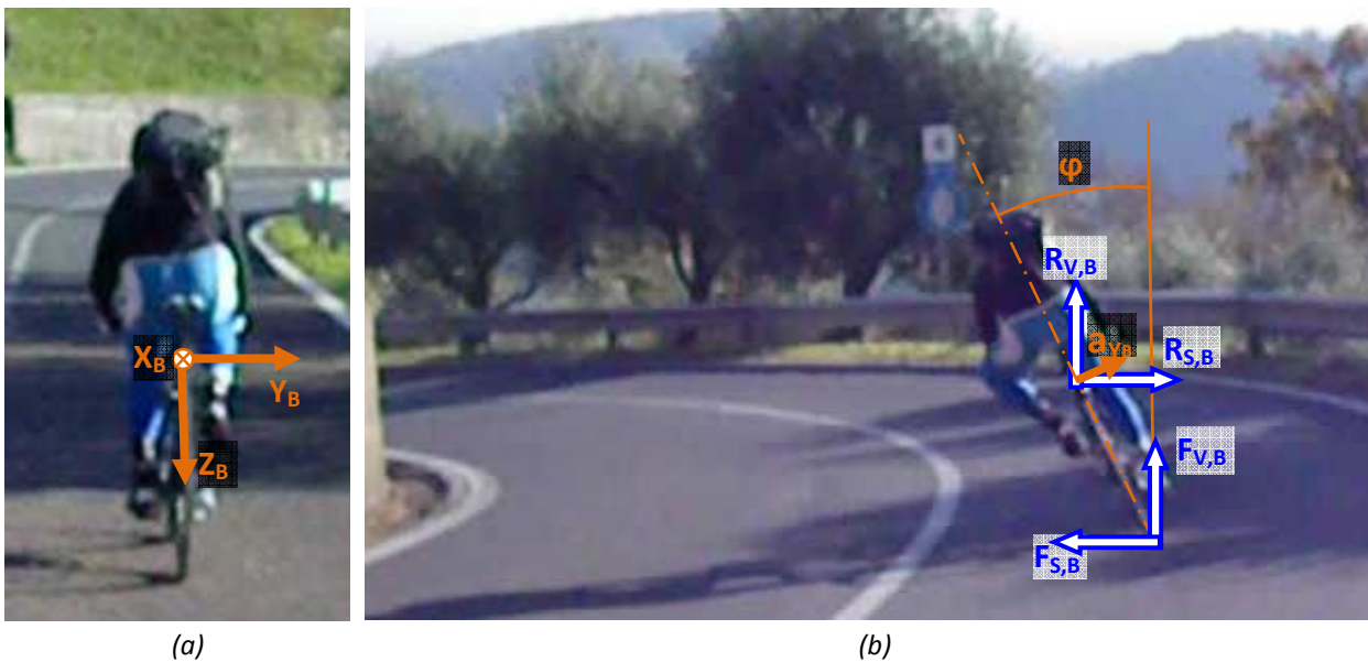
Fig. 13.5. (a) Reference system adopted for the bike; (b) acceleration along the Y B axis measured during the execution of a left curve.
