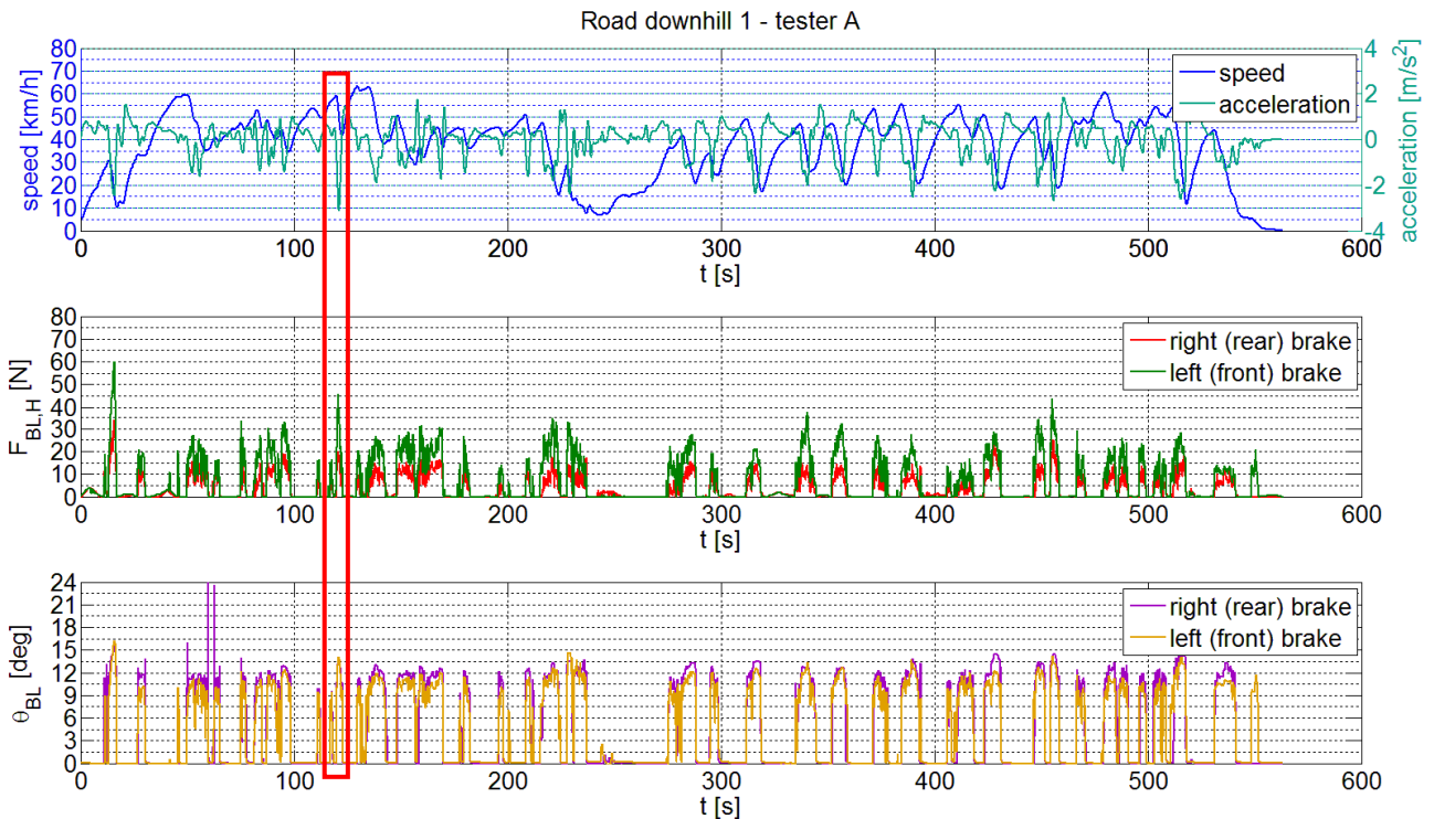
Fig. 18.10 Signals regarding the Road Downhill 1 performed by the Tester A and selection of the reference braking action.
