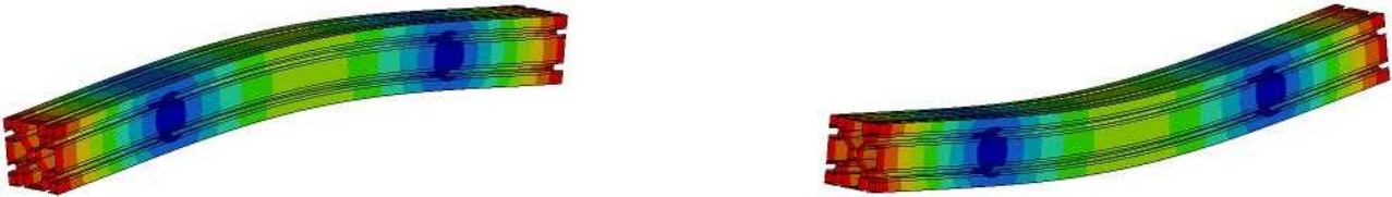
Fig. 5.18 First bending mode at 54 Hz of a 90x90 aluminium profile, 1 m long.
