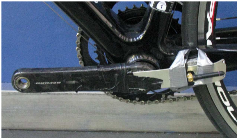
Fig. 17.5 Wireless transmitter of the strain gauge signal of the spider arm.
