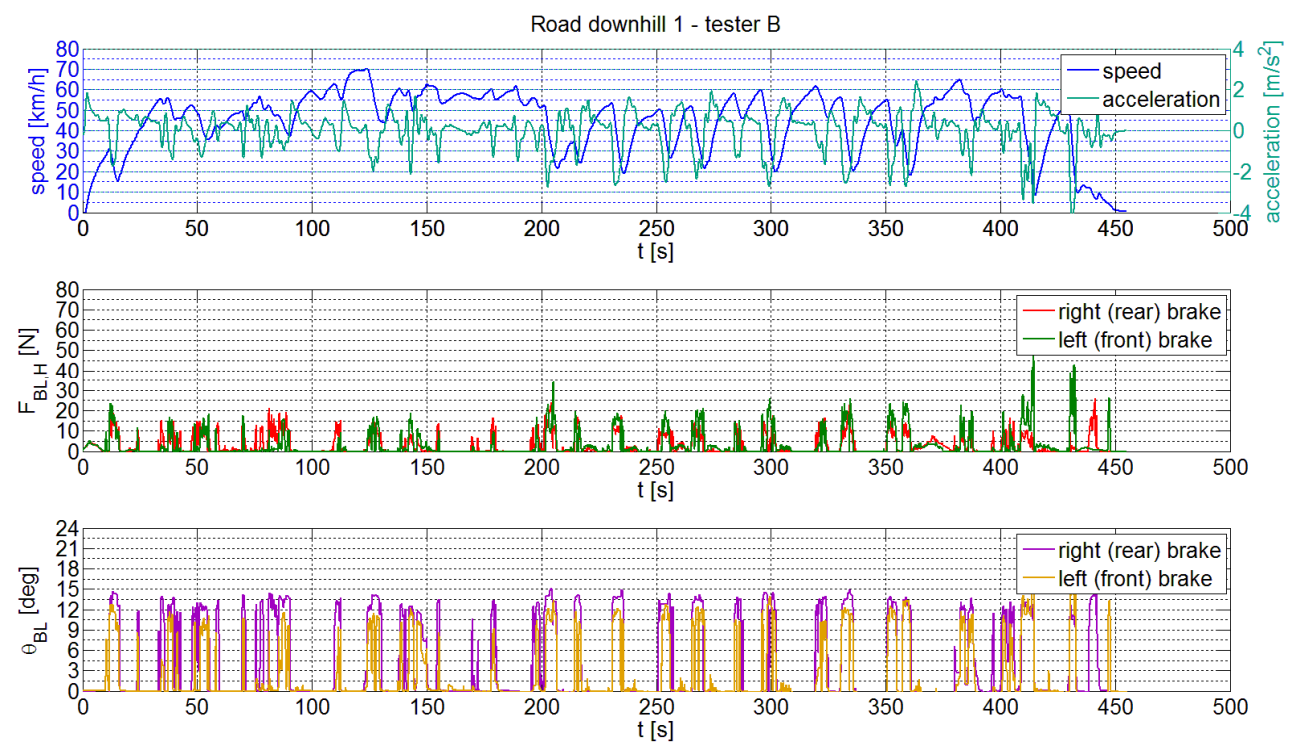
Fig. 18.8 Signals regarding the Road Downhill 1 performed by the Tester B.
