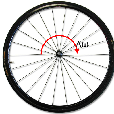
Fig. 12.3 Schematic of the wheel motion component, which causes the rotational kinetic energy increment.
