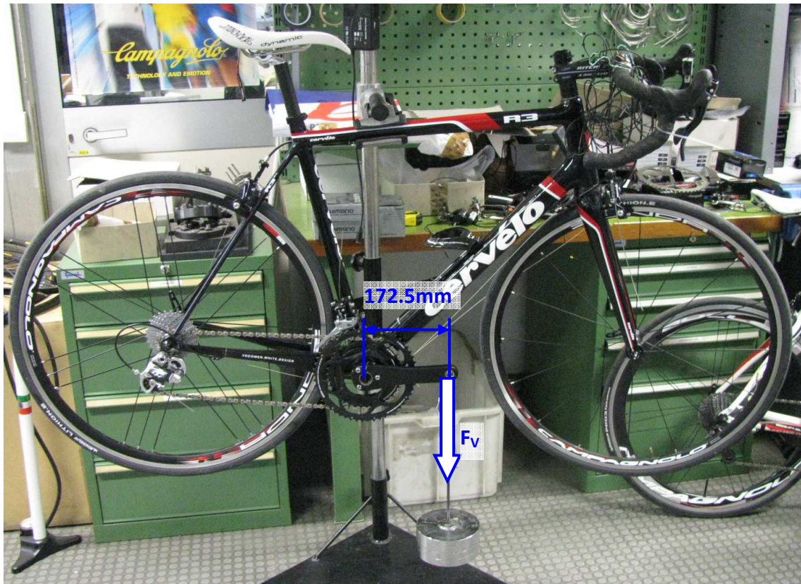
Fig. 17.16 Setup of the calibration test of the spider arm.
