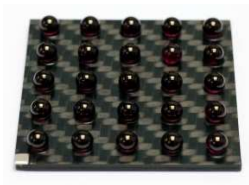
Figure 4.2: CT ball plate (spheres have a nominal diameter of 5 mm and are placed on a 5 x 5 grid with inter-sphere distance of 10 mm). [58]
