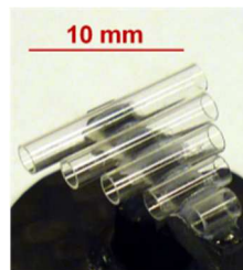
Figure 3.11: ‘Pan flute’ gauge consisting in 5 tube made by borosilicate glass with different calibrated lengths [43].
