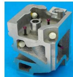
Figure 3.12: Aluminum segment dismountable freeform reference standard developed by PTB [56]
