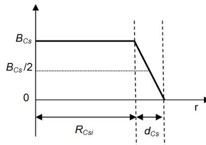
Figure 5.6: Magnetic flux pattern in the central solenoid inner space and in the edge.
