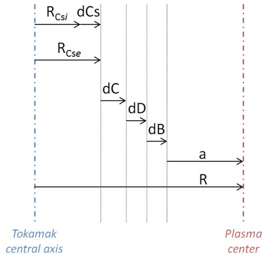
Figure 5.1: Radial inboard *unscaled* extension of a tokamak as modelled in FRESKO. It must be underlined that  $dB$  is obtained by the sum of shields, manifolds and first wall thickness).
