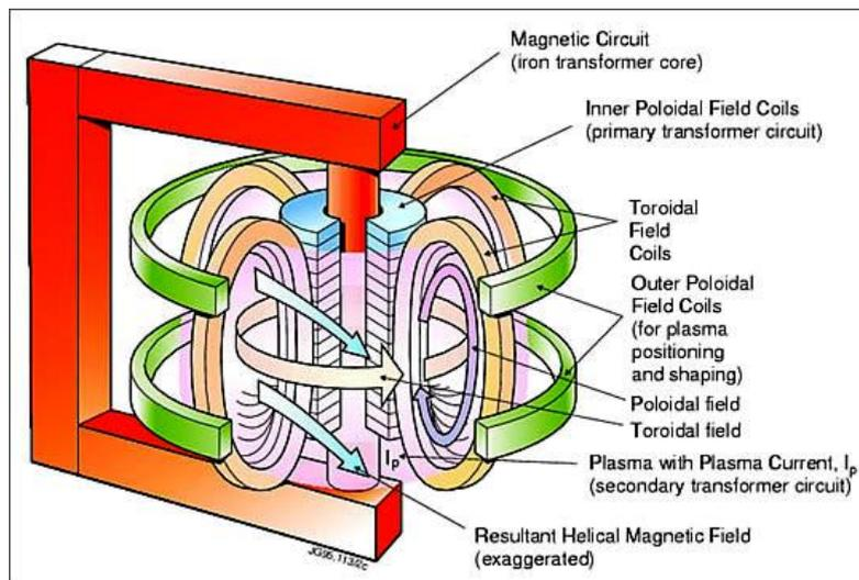
Figure 4.3: The principle magnetic circuits of JET's Tokamak
