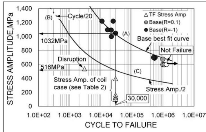
Figure 5.10: “S–N curve of JJ1 base metal at 4.2 K. The TF coil case stress amplitude includes the residual stress of 50 MPa. Curve (A) is the best-fit S–N curve using Eq. (1). Design S–N curve consist of curves (B and C).” [Hamada,2005]
