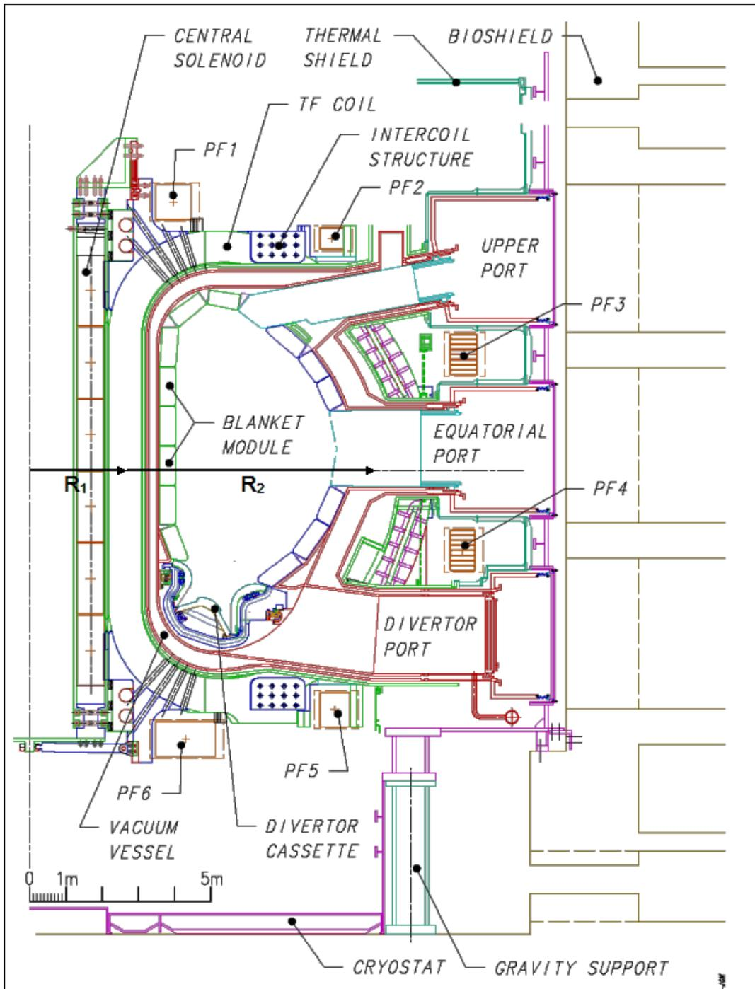
Figure 5.4: ITER tokamak cross section: the image is taken from [FDR,2001] and modified in order to highlight  $R_1$  and  $R_2$ .
