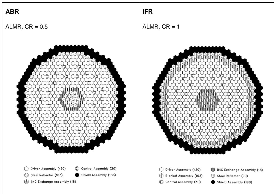
Figure 6.7: Geometry of a breeding ratio 0.5 and 1 core of an advanced liquid metal reactor.
