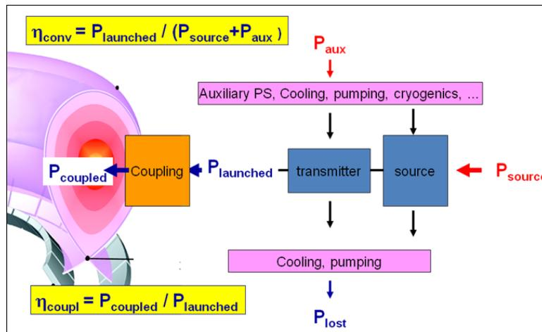
Figure 5.7: Auxiliary heating conversion and coupled efficiency definition, from [Pamela,2009].
