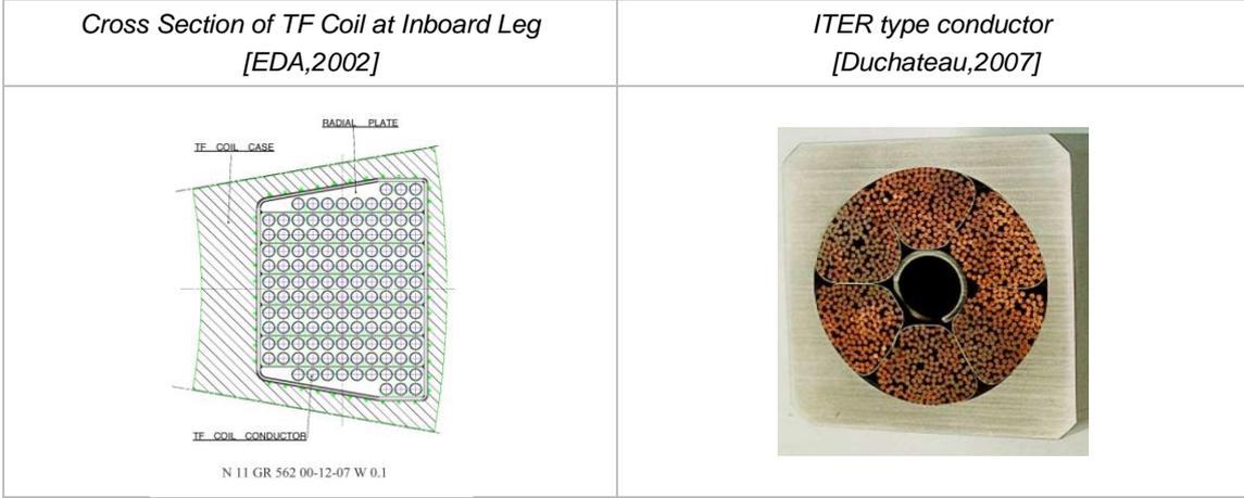
Figure 5.3: The TF coils consist of a winding pack contained in a thick steelcase (image on the left) The winding pack is a bonded structure of radial plates (which contain the conductor) with an outer ground insulation. The winding pack design is based on the use of Nb3Sn-type superconductor [Mitchell,2009] (image on the right) supported by radial plates. This design has advantages in terms of the conductor insulation, long-term quality, and reliability. [EDA,2002]
