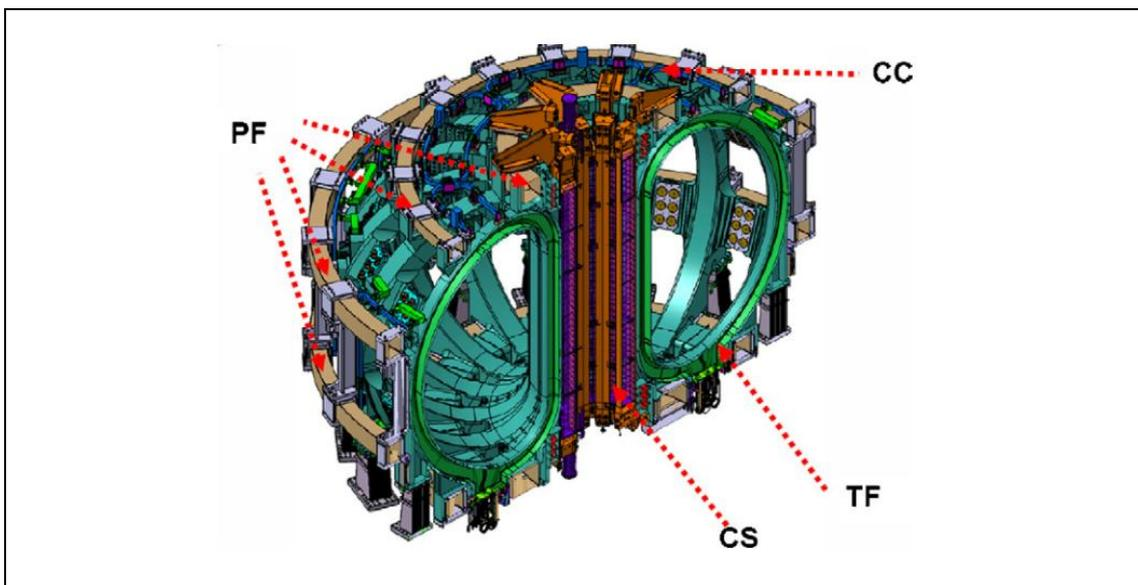
Figure 5.9: Main components of ITER magnet systems [Mitchell,2009]
