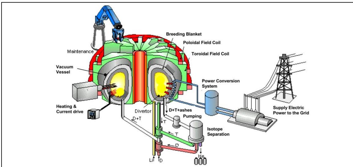
Figure 4.4: Schematic diagram of a tokamak fusion power station.
