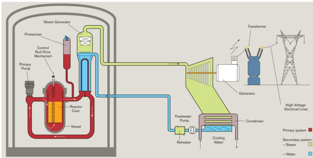
Figure 4.2: Simplified scheme of a PWR: the use of two separated system for heating exchange is highlighted. [Areva,2009]
