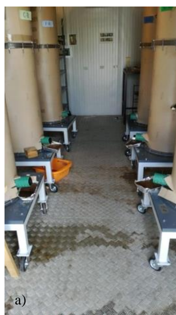
Figure 1. Set up of the semi-aerobic landfilling reactors (a) and constructive details of the individual reactors (b). The lengthening of columns to enable conduction of the second research phase is indicated.
