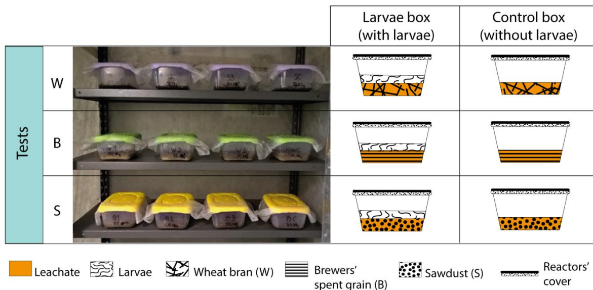
Figure 1. Experimental set up of the tests and research program. Materials and substrate typologies are graphically indicated.
