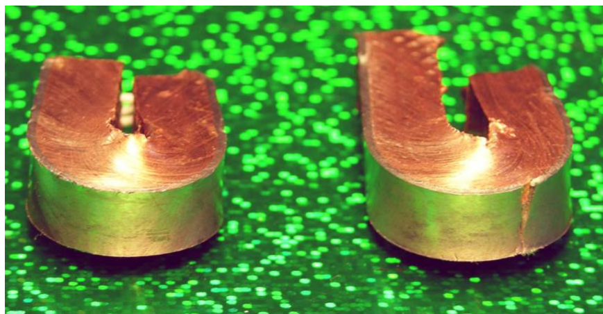
Figure 3.20: Bend tests - the samples were 150° bent, without cracking.
