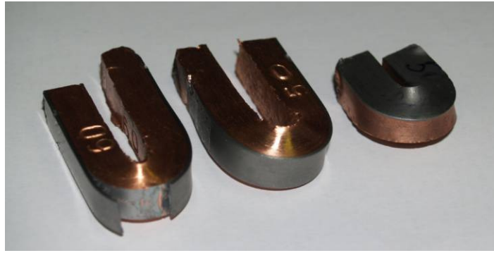
Figure 3.50: bend test specimens: they were 150° bent, without cracking; a crack appeared and developed in delamination in the transverse sample (left) after further bending, up to 180°
