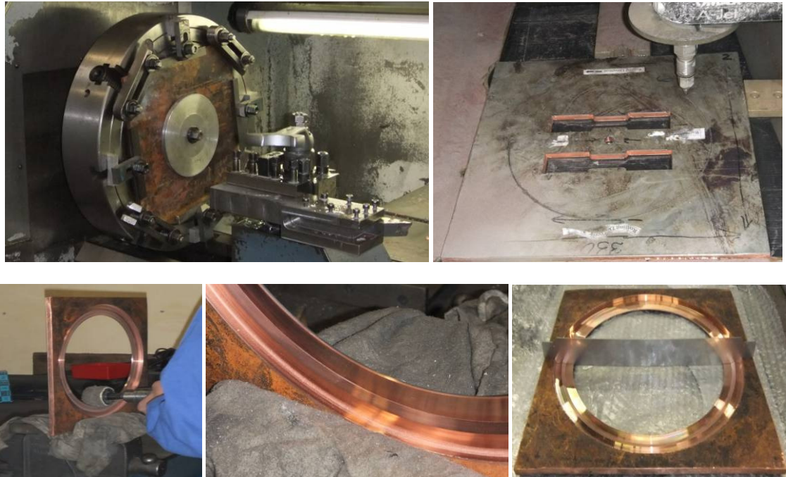
Figure 3.59: Preparation of samples for pressing. Top left: tight fixing in lathe. Top right: water-jet cutting of inner circle (and tensile test specimens). Bottom left: polishing of the finger tip. Bottom middle: close up of the finger. Bottom right: control of the shape of the finger with a laser cut jig
