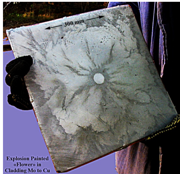
Figure 3.19: Explosive bonded prototype. Note the unbounded center; this was the ignition point. The ‘flower-like’ appearance is from detonation products and was removed by cleaning
