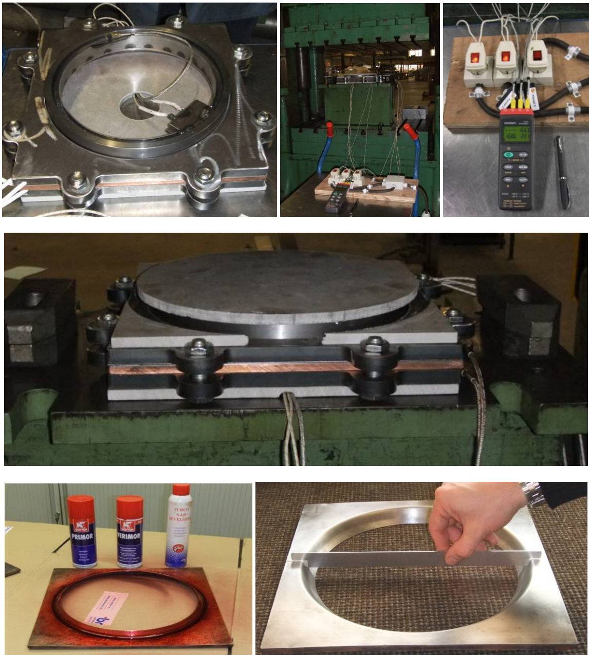
Figure 3.60: The forming step of the plates. Top row: Left-assembled tooling; Middle-ready for pressing; Right-temperature measurement and switches for the 3 tooling parts. Middle row: assembled tooling with insulating material. Bottom row: Left-penetrant test; Right-checking the diameter of 275mm at 11.5 mm depth, with the laser cut jig
