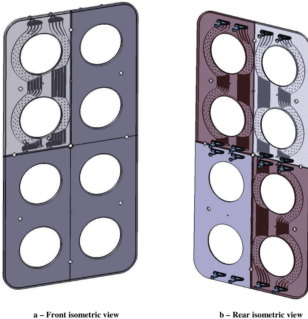
Figure 2.11: Front and rear isometric views of the MITICA Plasma Drivers Plate
