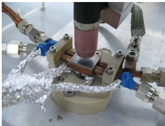
a – view of the specimen after pulse 15000
