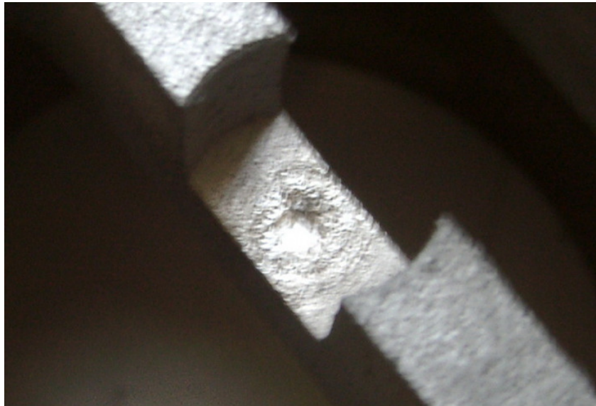
Figure 2.5: Three millimeters erosion area of Mo target during tests performed at BINP.
