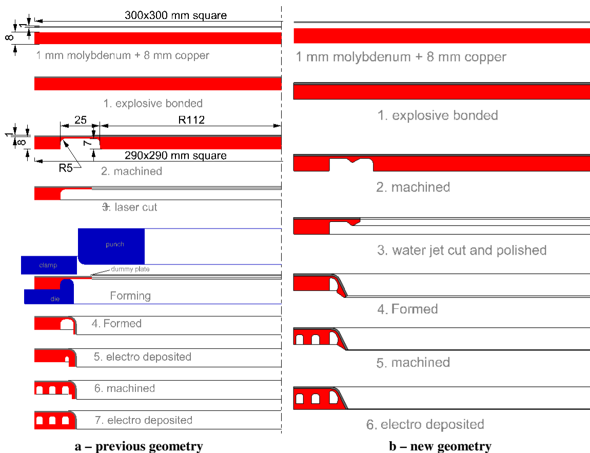
Figure 3.61: Driver hole rim geometries and manufacturing steps
